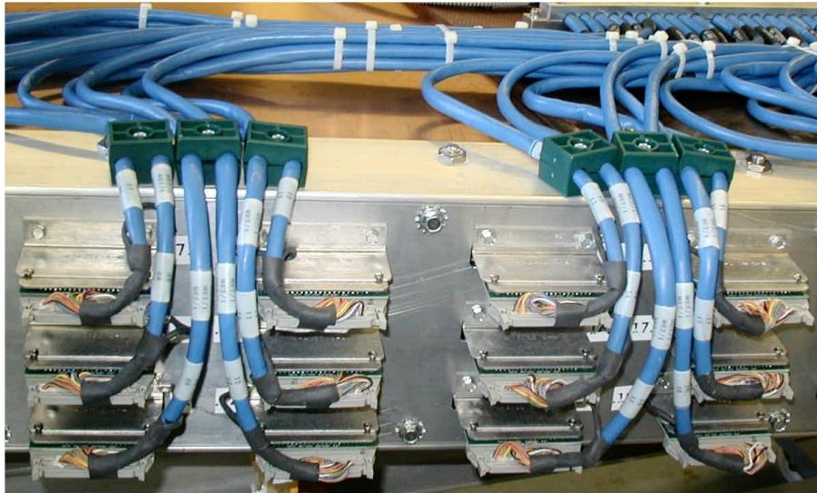
Figure 5: A view of the anode front-end boards installed on a chamber. Also shown are the AFEBoard-ALCT cables.
