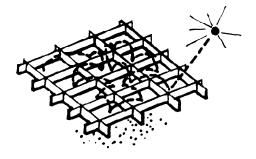
The second factor entering into the non-leakage term is related to the size and shape of the reactor, only. It is possible to combine all pertinent information on size and shape in a single expression. This turns out to vary inversely as the second power of the characteristic dimensions of the reactor. It is called the geometric buckling,  $B_g^2$ . Formulae for the geometric buckling of the simplest shapes are as follows:
