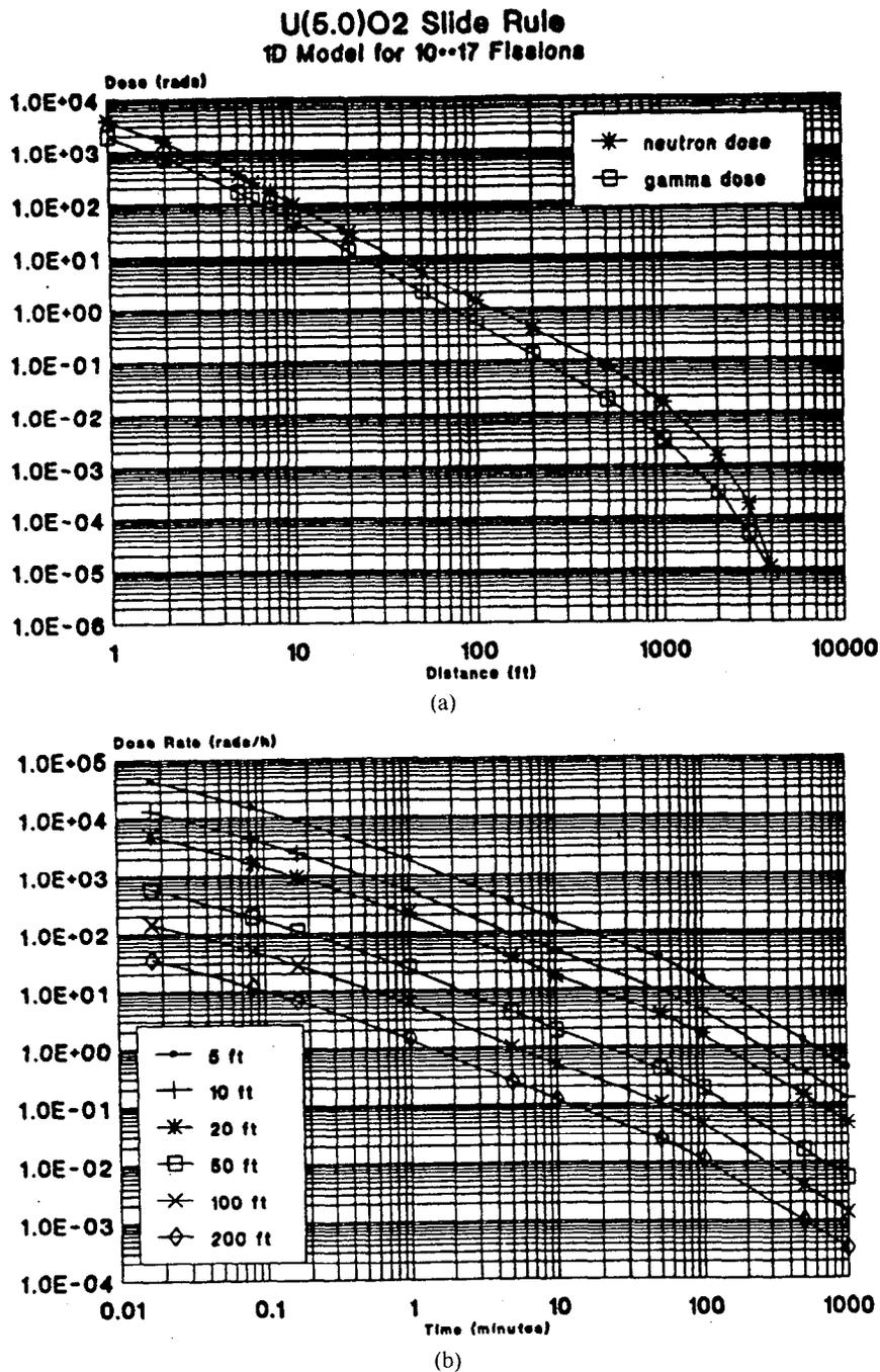
Fig. 2. Slide rule for U(5.0)O<sub>2</sub>: (a) prompt dose as a function of distance and (b) fission product gamma dose rate as a function of elapsed time.
