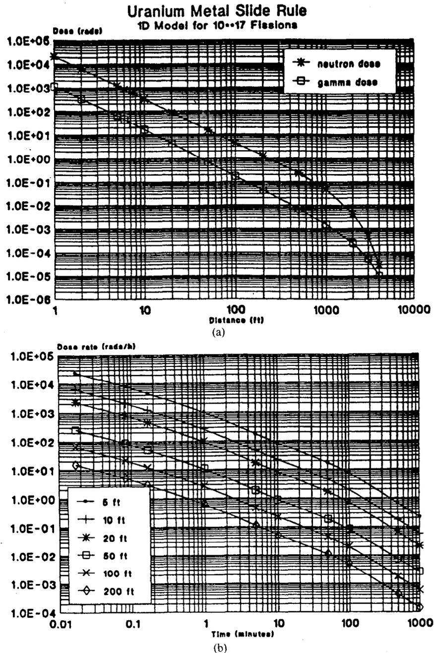
Fig. 1. Slide rule for U(93.2) metal: (a) prompt dose as a function of distance and (b) fission product gamma dose rate as a function of elapsed time.
