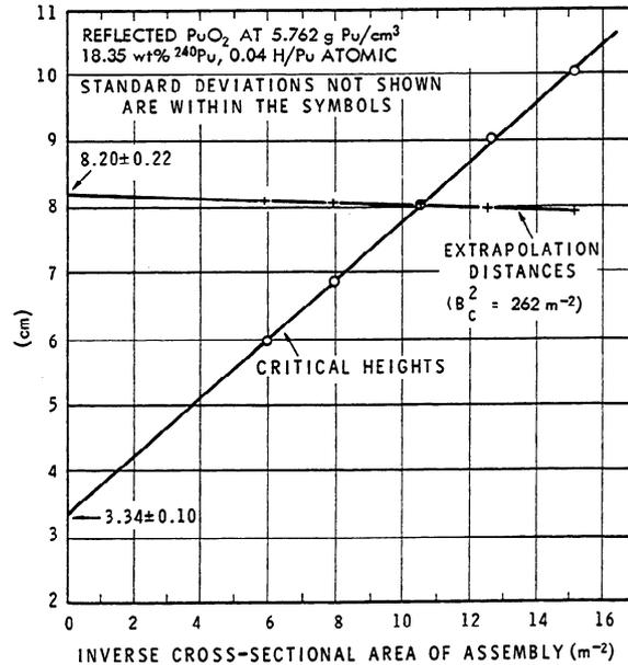
Fig. 1. Extrapolation distances and measured critical height.
