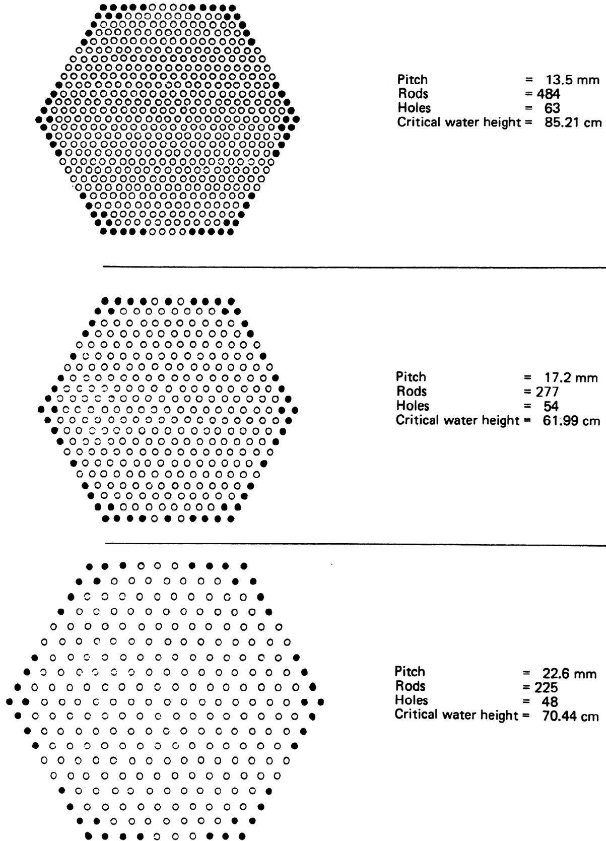
Fig. 5. Diagram of the three pseudo-cylindrical configurations. Rods = white dots; holes = black dots.
