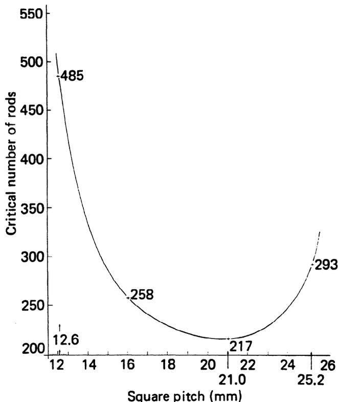
Fig. 4. Curve giving the critical number of completely immersed rods as a function of the pitch of a square lattice.
