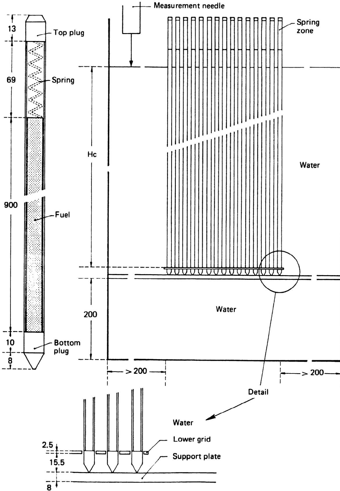
Fig. 1. Principal dimensions of the fuel rods and their assembly (in millimetres).
