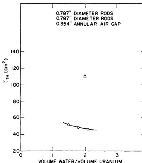
Figure 3a.  $\tau_{th}$  vs volume ratio, 0.787 inch (2.00 cm) diameter natural uranium rods in light water. From 1944-45 Oak Ridge experiments
