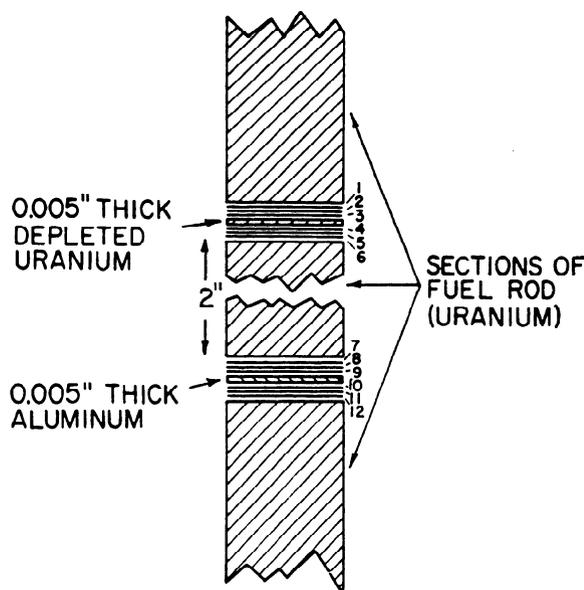
Figure 8. Schematic arrangement of fuel rod and uranium and aluminum foil used to measure fast effect
