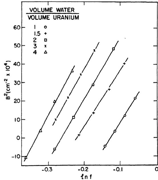
Figure 19.  $\ln f$  vs  $B^2$  for boron poisoned lattices of 0.600 inch diameter, 1.143% enriched uranium rods in light water
