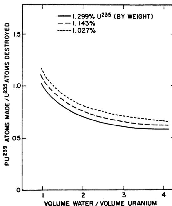
Figure 22. Conversion ratio of 0.600 inch diameter, slightly enriched uranium rod lattices in light water
