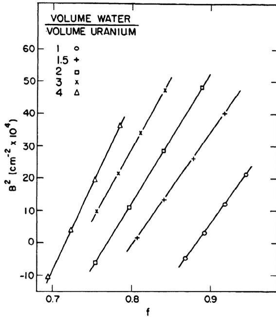
Figure 18.  $f$  vs  $B^2$  for boron poisoned lattices of 0.600 inch diameter, 1.143% enriched uranium rods in light water
