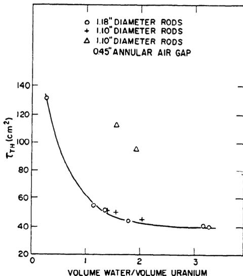
Figure 3.  $\tau_{th}$  vs volume ratio, 1.10 inch and 1.18 inch diameter natural uranium rods in light water. From 1944-45 Oak Ridge experiments
