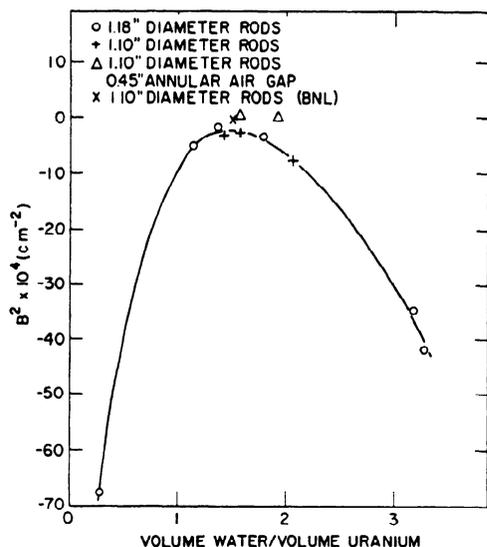
Figure 1.  $B^2$  vs volume ratio, 1.10 inch and 1.18 inch diameter natural uranium rods in light water. From 1944-45 Oak Ridge experiments
