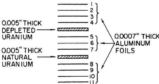
Figure 10. Schematic of uranium-aluminum sandwich used in fast-effect calibration experiment
