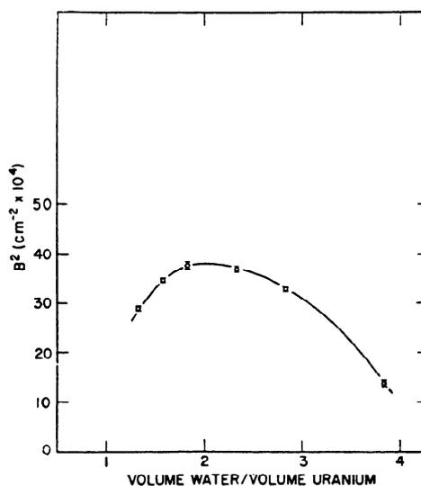
Figure 5. Experimental values of buckling for 0.750 inch diameter, 1.027% enriched uranium rods in light water
