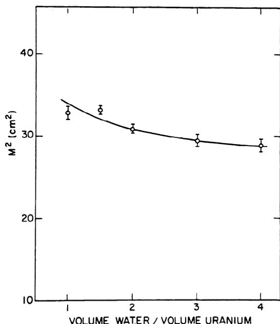
Figure 20. Best values of migration areas of fission neutrons in lattices of 0.600 inch diameter, slightly enriched uranium rods and light water
