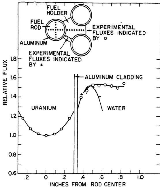
Figure 16. Experimental intracell flux traverse, 0.600 inch diameter, 1.143% enriched uranium rods in light water. Volume ratio = 1.5:1
