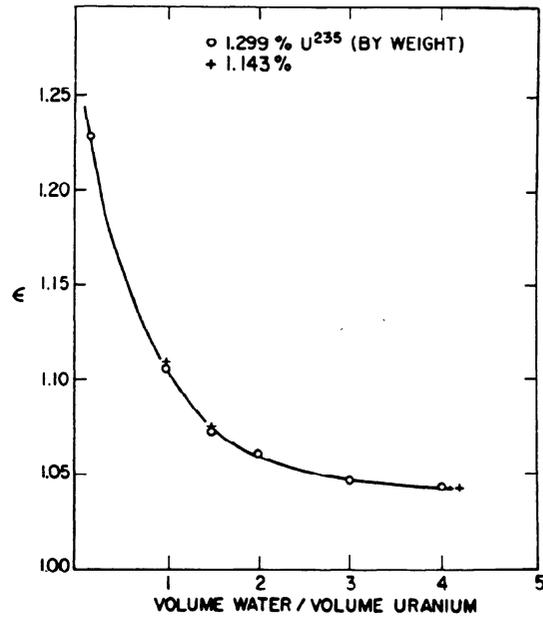
Figure 15. Experimental fast effect of 0.600 inch diameter, slightly enriched uranium rods in light water
