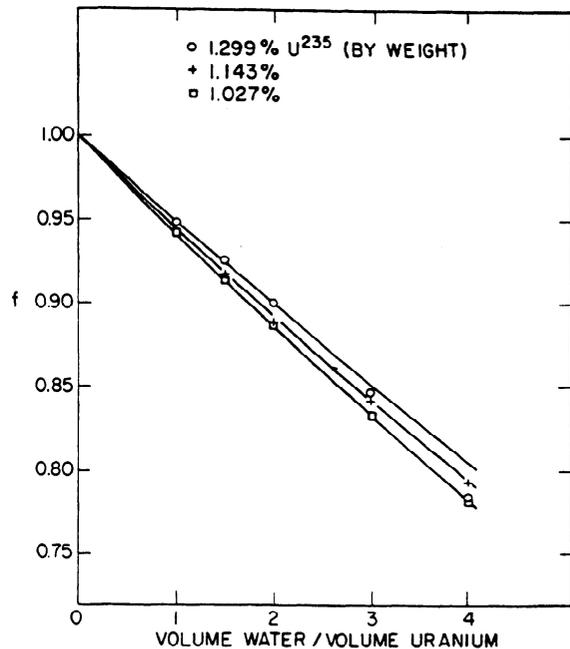
Figure 17. Measured thermal utilization, 0.600 inch diameter, slightly enriched uranium rods in light water
