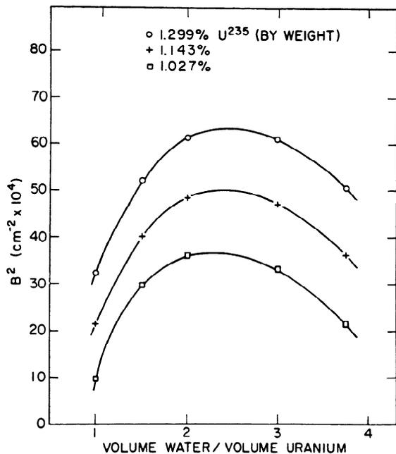
Figure 13. Experimental values of buckling, 0.600 inch diameter, slightly enriched uranium rods in light water
