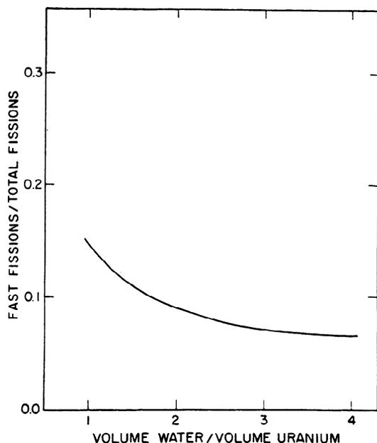
Figure 21. Experimental fast fission fraction for 0.600 inch diameter uranium rod lattices in light water
