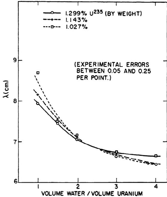
Figure 14. Reflector savings of 0.600 inch diameter, slightly enriched uranium rods in light water
