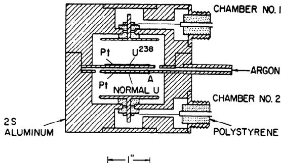
Figure 9. Fission chamber used for fast effect calibration experiment
