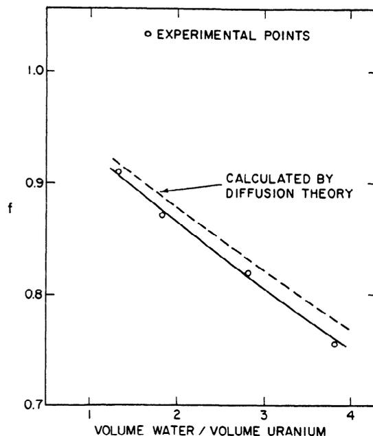
**Figure 11. Thermal utilization of 0.750+ inch diameter, 1.027% enriched uranium rods in light water**
