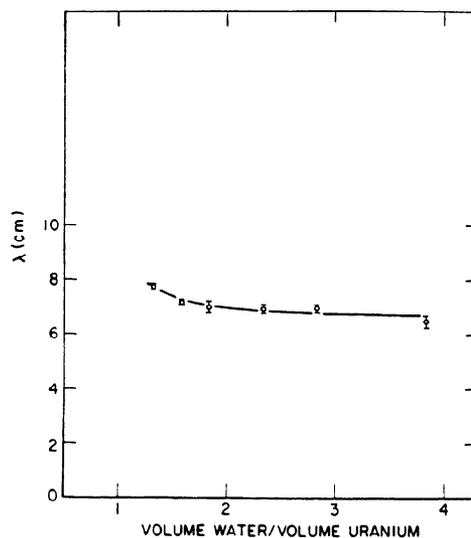
Figure 6. Experimental values of reflector savings for 0.750 inch diameter, 1.027% enriched uranium in light water
