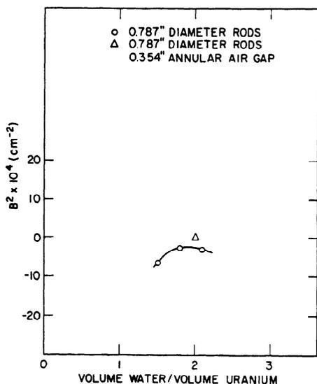
Figure 2.  $B^2$  vs volume ratio, 0.787 inch diameter natural uranium rods in light water. From 1944-45 Oak Ridge experiments
