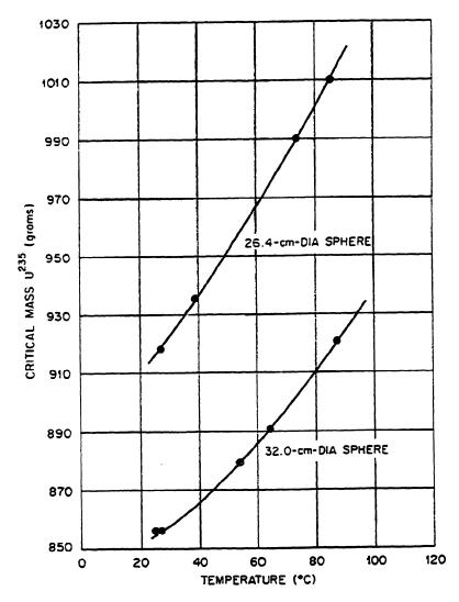
FIG. 5. Critical mass of U<sup>235</sup> in water-reflected spherical reactors as a function of temperature.
