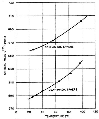
FIG. 6. Critical mass of U<sup>233</sup> in water-reflected spherical reactors as a function of temperature.
