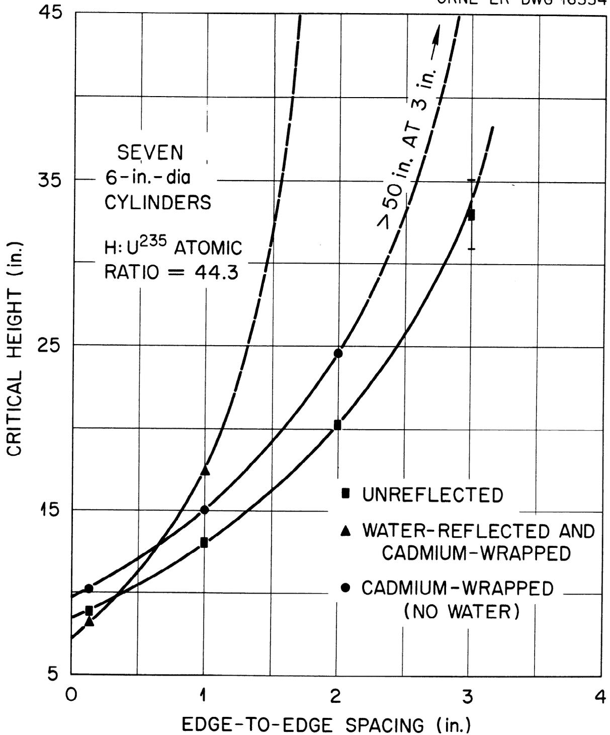
Fig. 4. Critical Height as a Function of the Edge-to-Edge Spacing of Unreflected and Water-Reflected 6-in.-dia Aluminum Cylinders Containing an Enriched  $U^{235}$  Solution: Hexagonal Arrays, With and Without Cadmium Wrapping.
