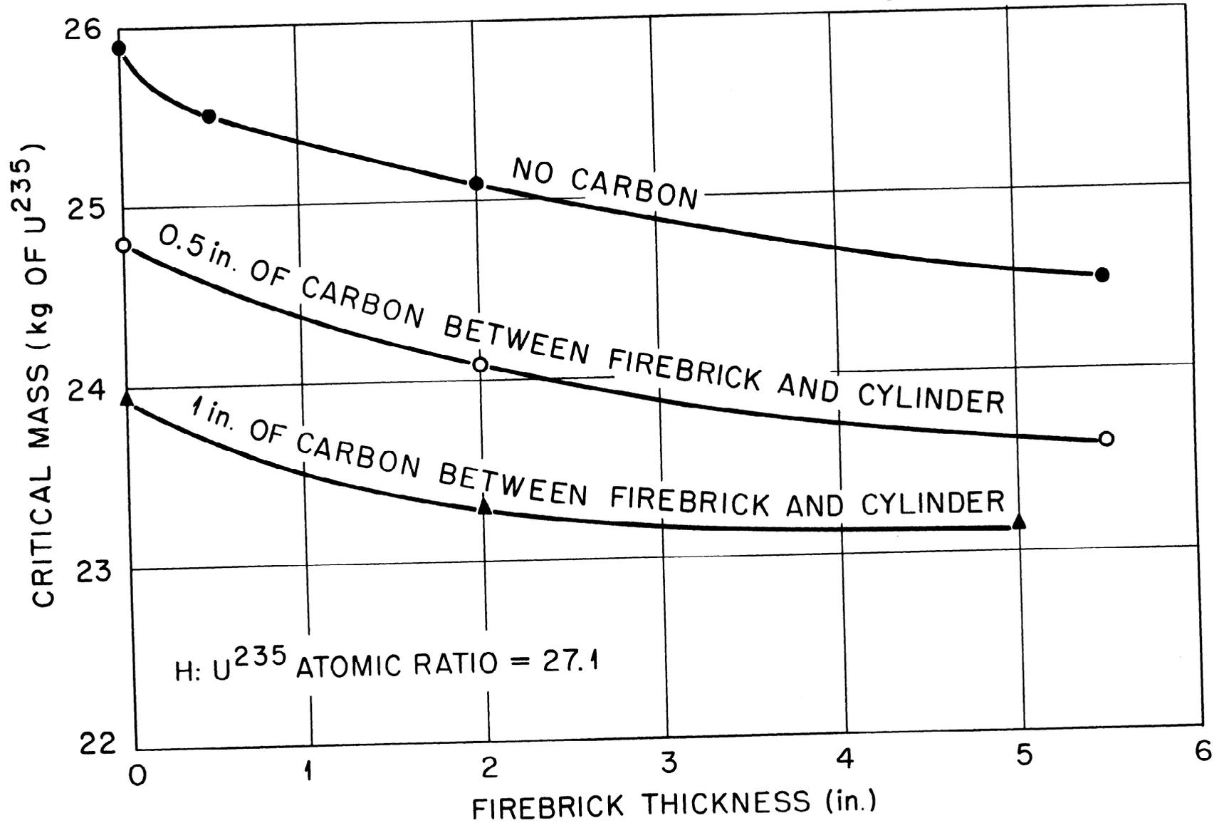
Fig. 21. Critical Mass as a Function of the Thickness of Carbon and Firebrick on the Bottom of a 20-in.-dia Aluminum Cylinder Containing an Enriched U<sup>235</sup> Solution.
