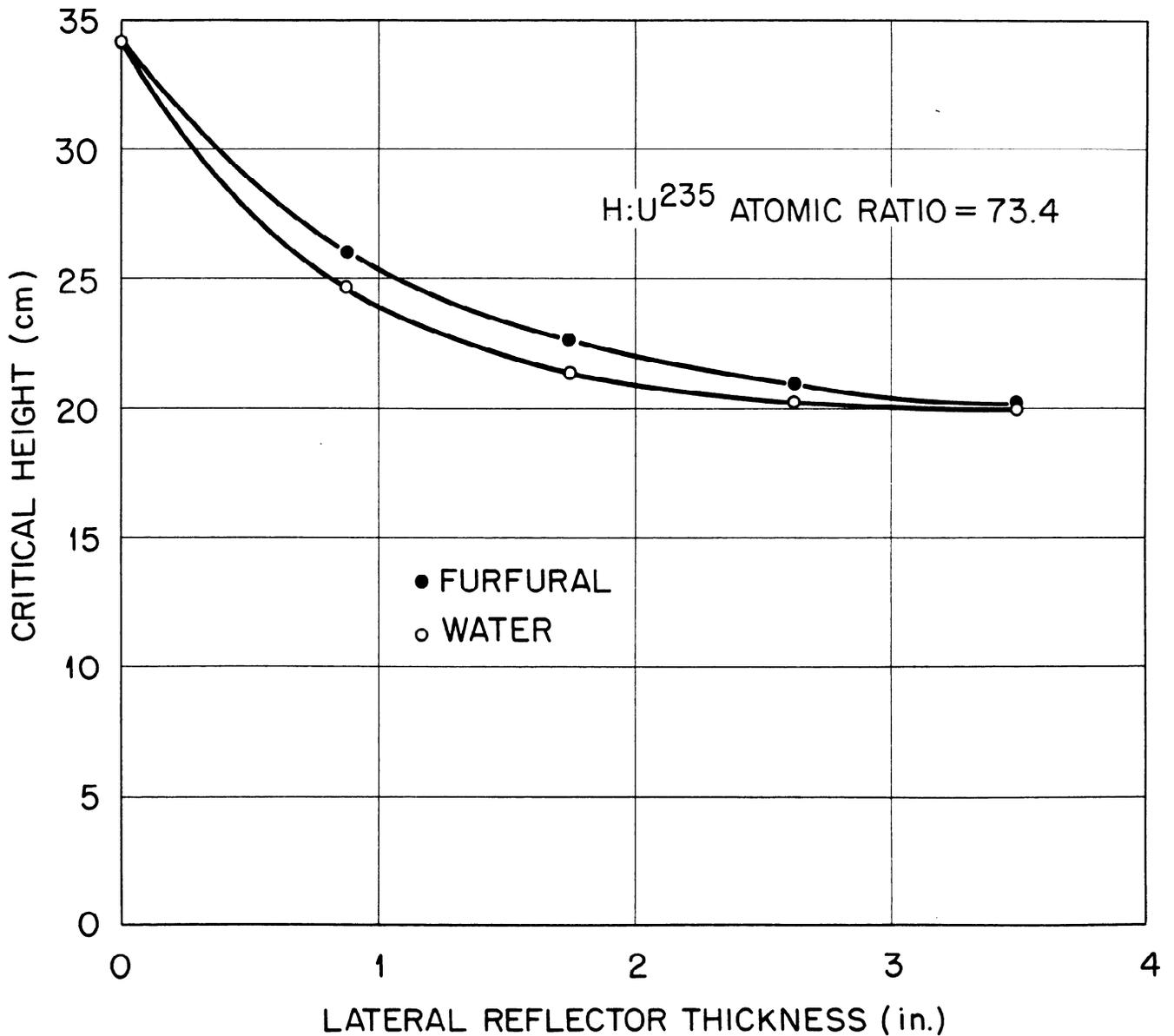
Fig. 19. Critical Height as a Function of the Thickness of a Water or Furfural Reflector on the Lateral Surface of a 10-in.-dia Aluminum Cylinder Containing an Enriched U<sup>235</sup> Solution.
