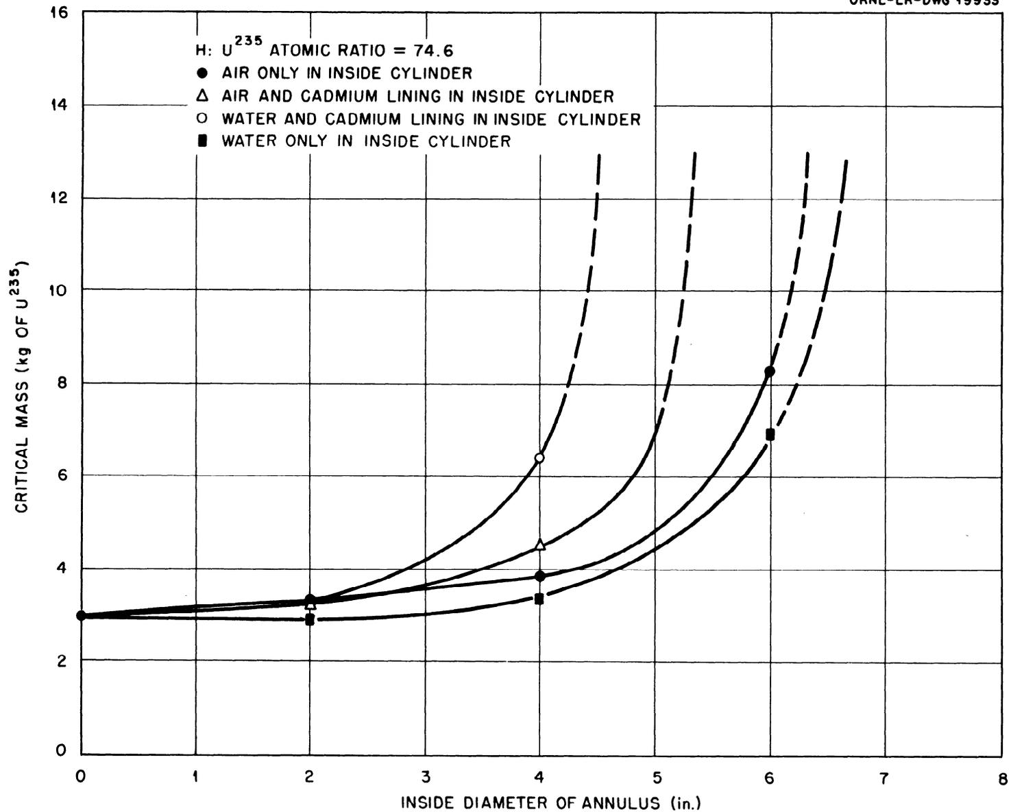
Fig. 18. Critical Mass as a Function of the Inside Diameter of a Water-Reflected 10-in.-OD Annulus Containing an Enriched  $U^{235}$  Solution; Inside Cylinder Filled with Air, or Water, with and without Cadmium Lining.
