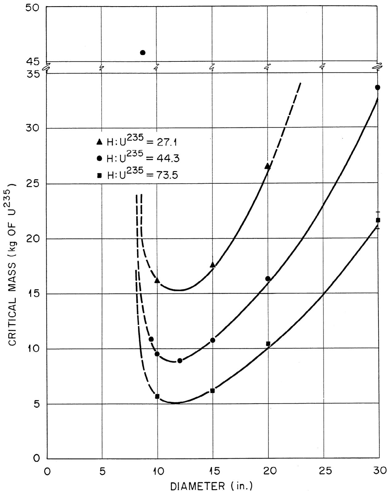
Fig.12. Critical Mass as a Function of the Diameter of Single Unreflected Aluminum Cylinders Containing Enriched U<sup>235</sup> Solutions.
