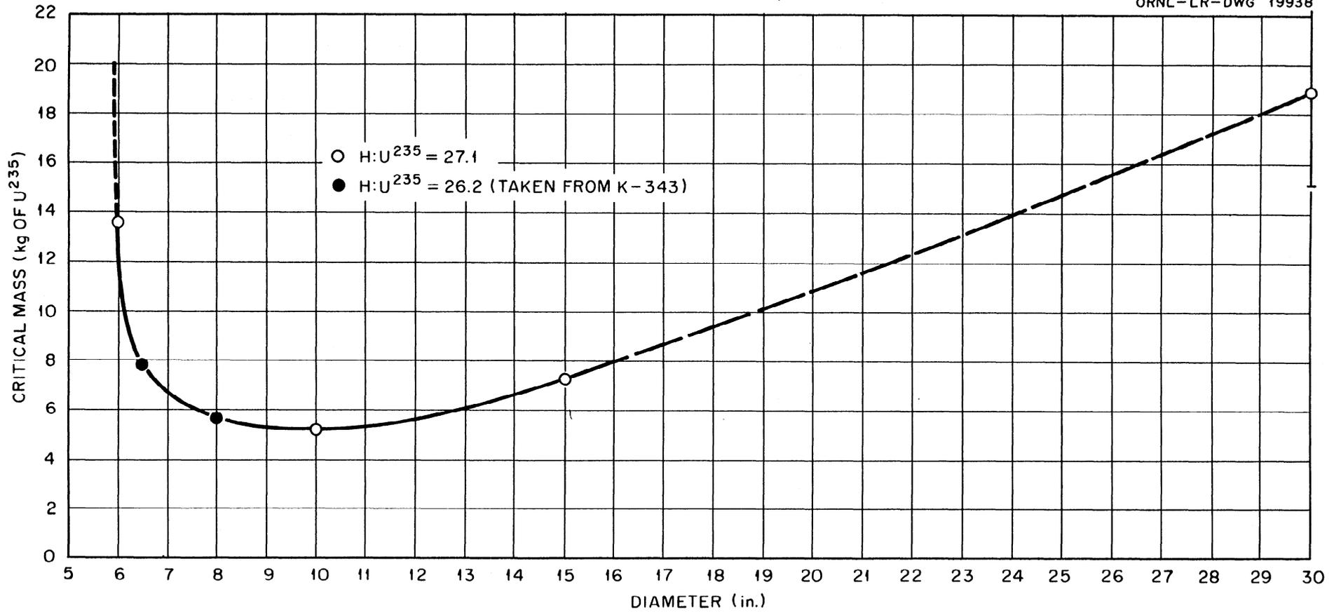
Fig. 11. Critical Mass as a Function of the Diameter of Single Water-Reflected Aluminum Cylinders Containing an Enriched U<sup>235</sup> Solution.
