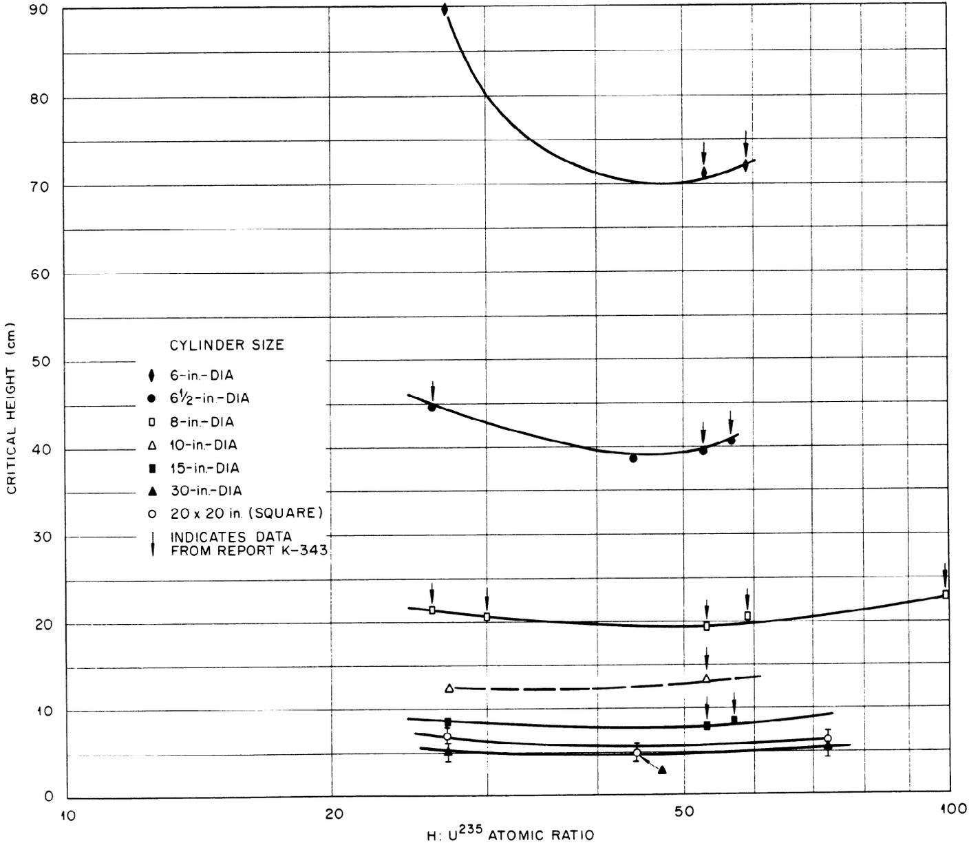
Fig. 13. Critical Height as a Function of the H: U<sup>235</sup> Atomic Ratio of Solutions Contained in Single Water-Reflected Aluminum Cylinders .
