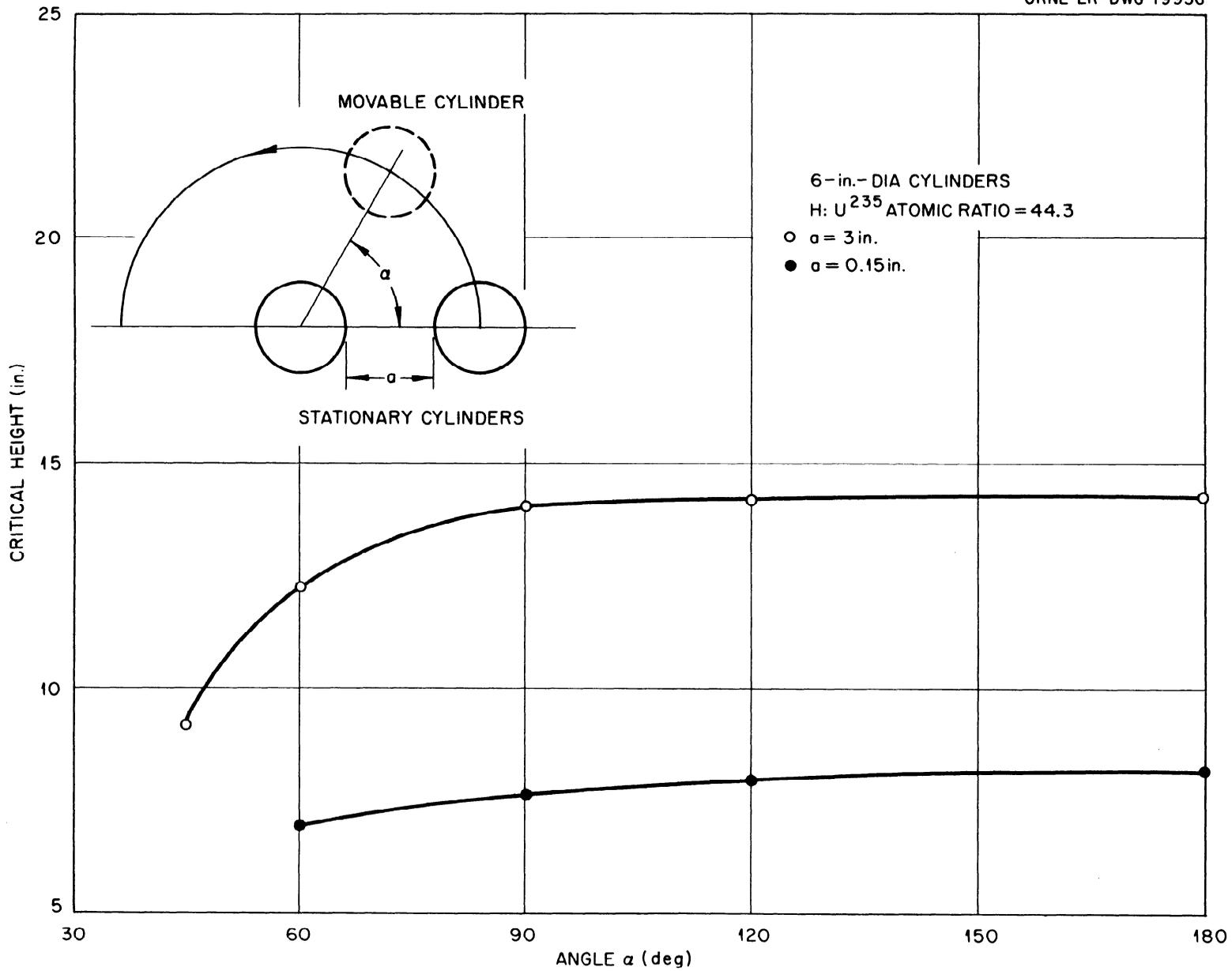
Fig. 8. Critical Height of Three Water-Reflected 6-in.-dia Aluminum Cylinders Containing an Enriched  $U^{235}$  Solution as a Function of the Vertex Angle of an Isosceles Triangle Describing the Relative Locations of the
