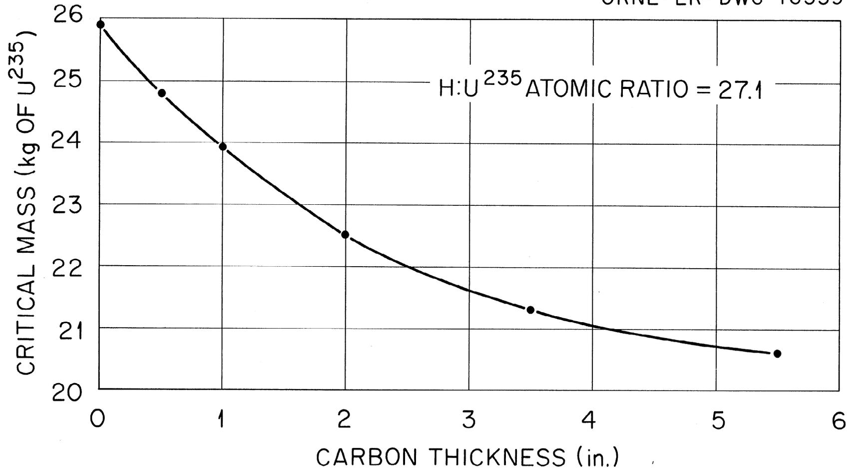
Fig. 22. Critical Mass as a Function of the Thickness of Carbon on the Bottom of a 20-in.-dia Aluminum Cylinder Containing an Enriched U<sup>235</sup> Solution.
