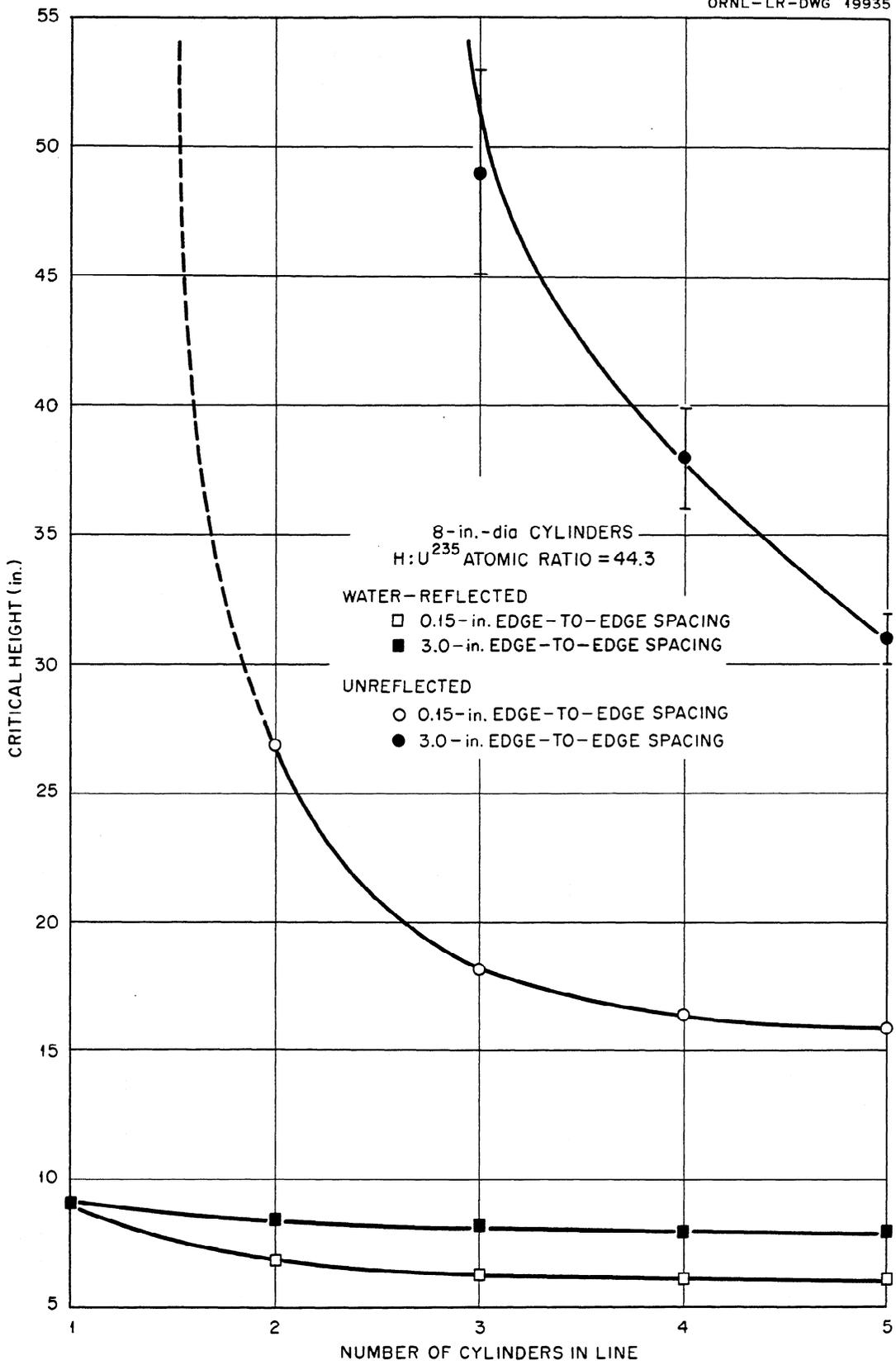
Fig. 7. Critical Height as a Function of the Number of Unreflected or Water-Reflected 8-in.-dia Aluminum Cylinders Containing an Enriched U<sup>235</sup> Solution. Straight-Line Arrays.
