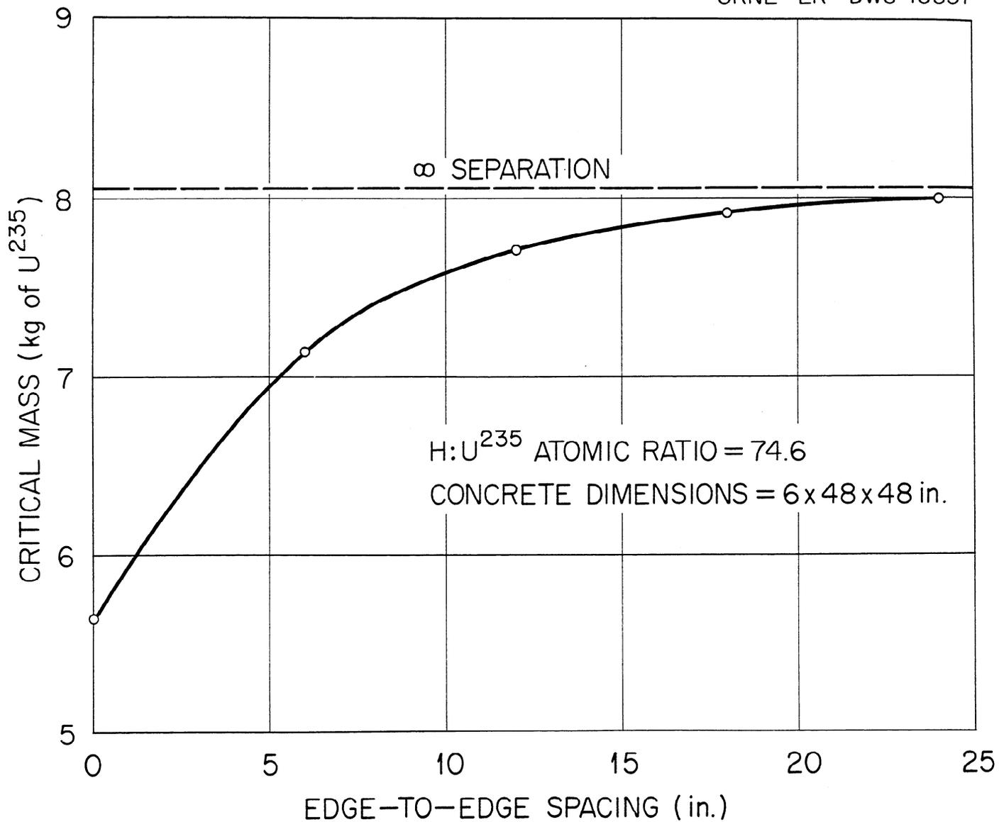
Fig. 20. Critical Mass as a Function of the Distance Between a 9-in.-dia Stainless Steel Cylinder Containing an Enriched U<sup>235</sup> Solution and a 6-in.-thick Concrete Wall.
