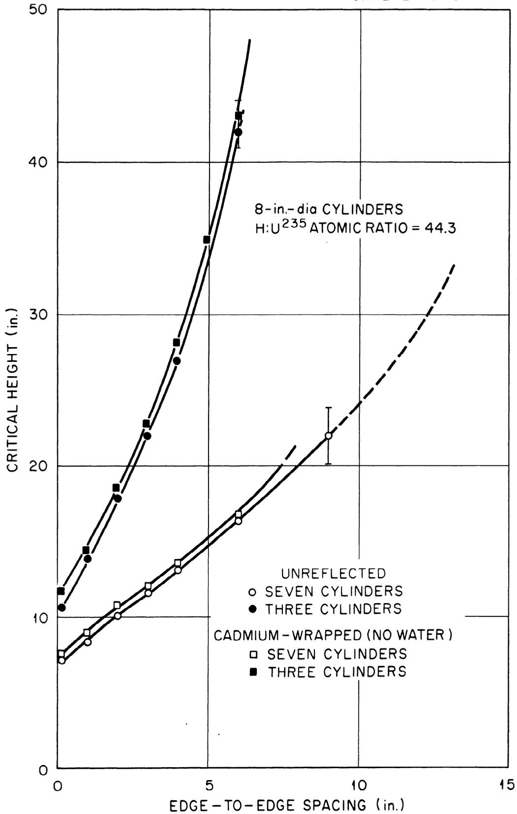
Fig. 5. Critical Height as a Function of the Edge-to-Edge Spacing of Unreflected 8-in.-dia Aluminum Cylinders Containing an Enriched U<sup>235</sup> Solution: Hexagonal and Triangular (Equilateral) Arrays, With and Without Cadmium Wrapping.
