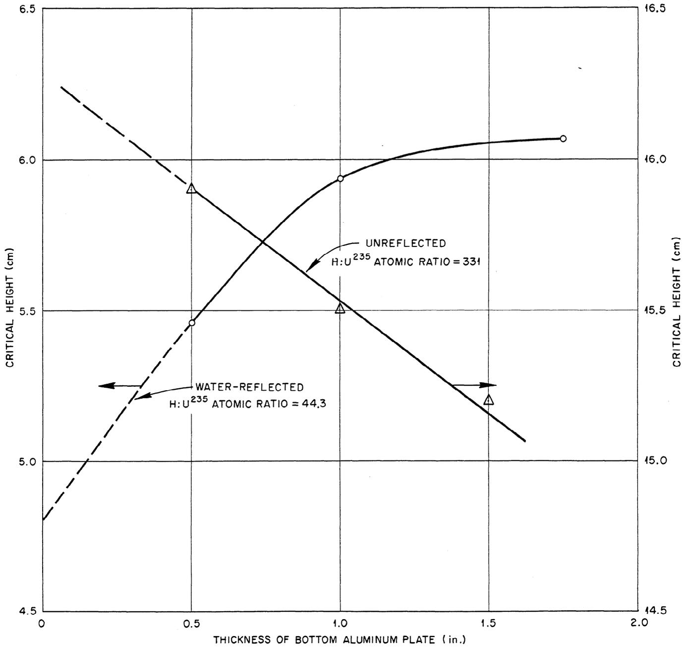
Fig. 16. Critical Height of an Enriched U<sup>235</sup> Solution Contained in a 30-in.-dia Aluminum Cylinder as a Function of the Thickness of the Cylinder Bottom Plate.
