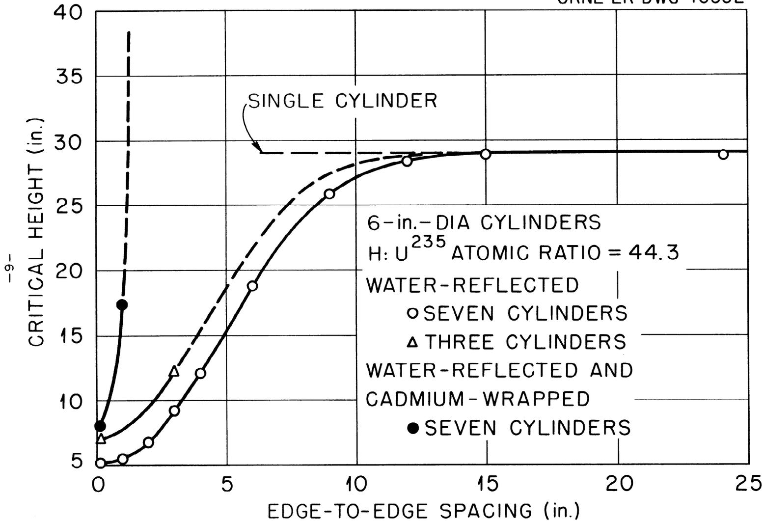
Fig. 2. Critical Height as a Function of the Edge-to-Edge Spacing of Water-Reflected 6-in.-dia Aluminum Cylinders Containing an Enriched U<sup>235</sup> Solution: Hexagonal and Triangular (Equilateral) Arrays, with and without Cadmium Wrapping.
