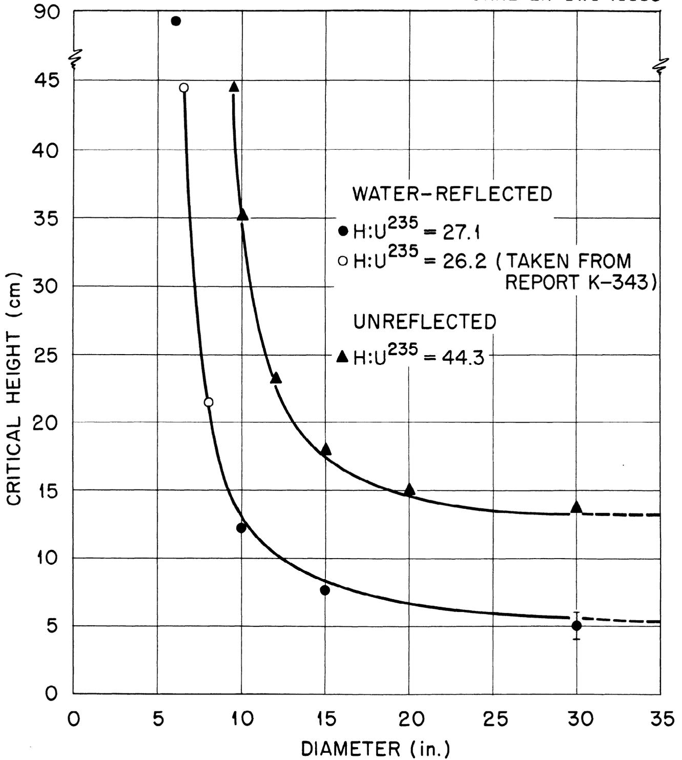
Fig. 10. Critical Height as a Function of the Diameter of Single Unreflected and Water-Reflected Aluminum Cylinders Containing Enriched U<sup>235</sup> Solutions.
