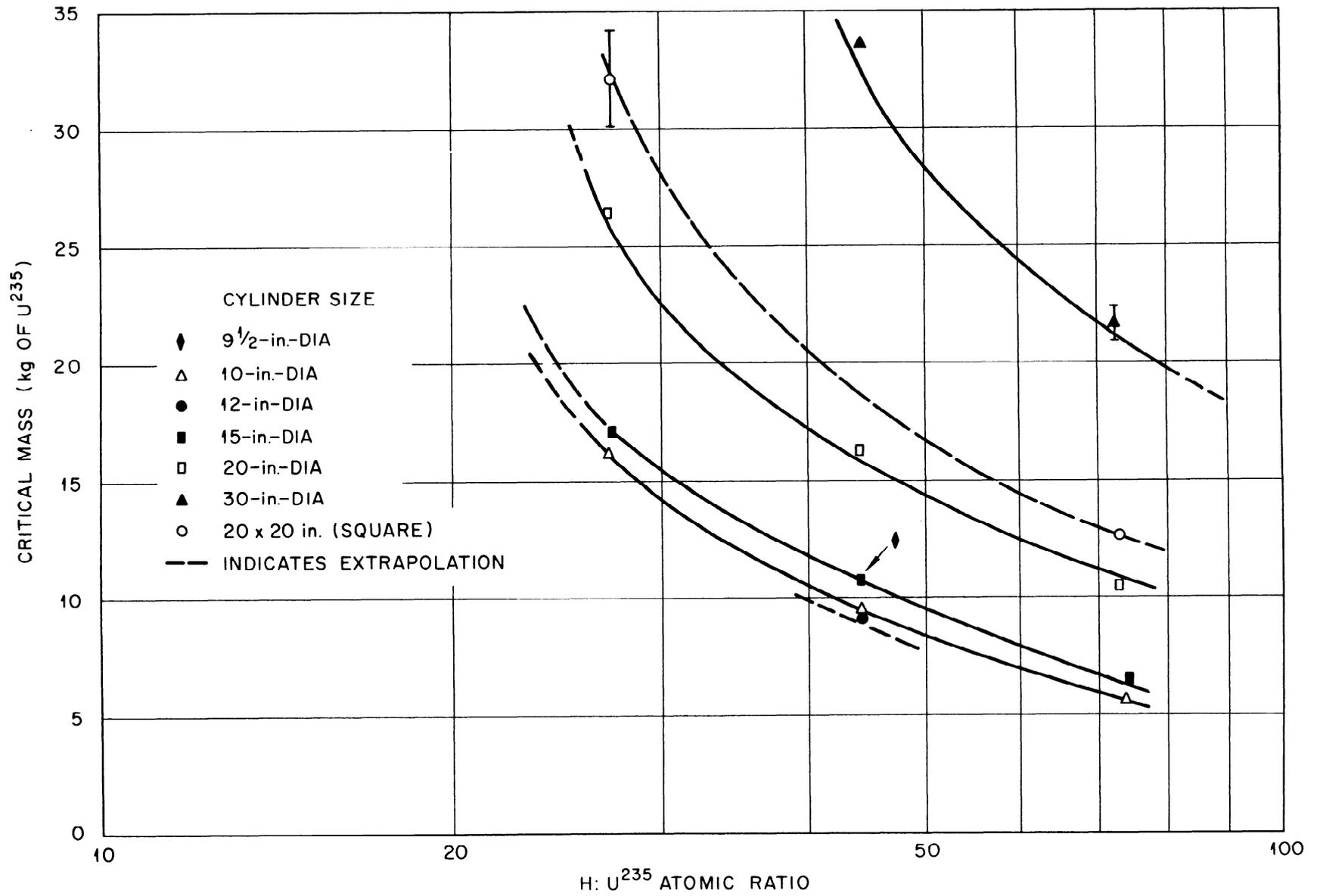
Fig. 15. Critical Mass as a Function of the H: U<sup>235</sup> Atomic Ratio of Solutions Contained in Single Unreflected Aluminum Cylinders.
