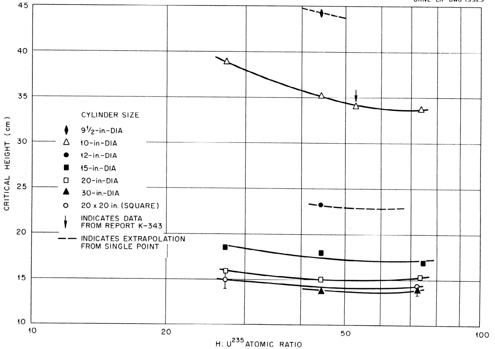
Fig. 14. Critical Height as a Function of the H:U<sup>235</sup> Atomic Ratio of Solutions Contained in Single Unreflected Aluminum Cylinders.
