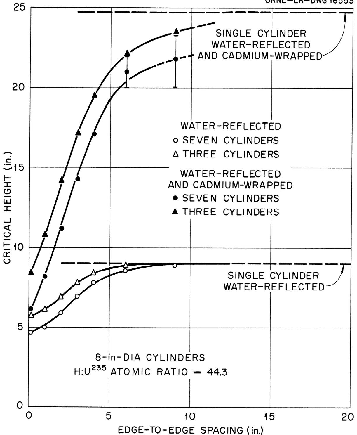
Fig. 3. Critical Height as a Function of the Edge-to-Edge Spacing of Water-Reflected 8-in.-dia Aluminum Cylinders Containing an Enriched U<sup>235</sup> Solution: Hexagonal and Triangular (Equilateral) Arrays, With and Without Cadmium Wrapping.
