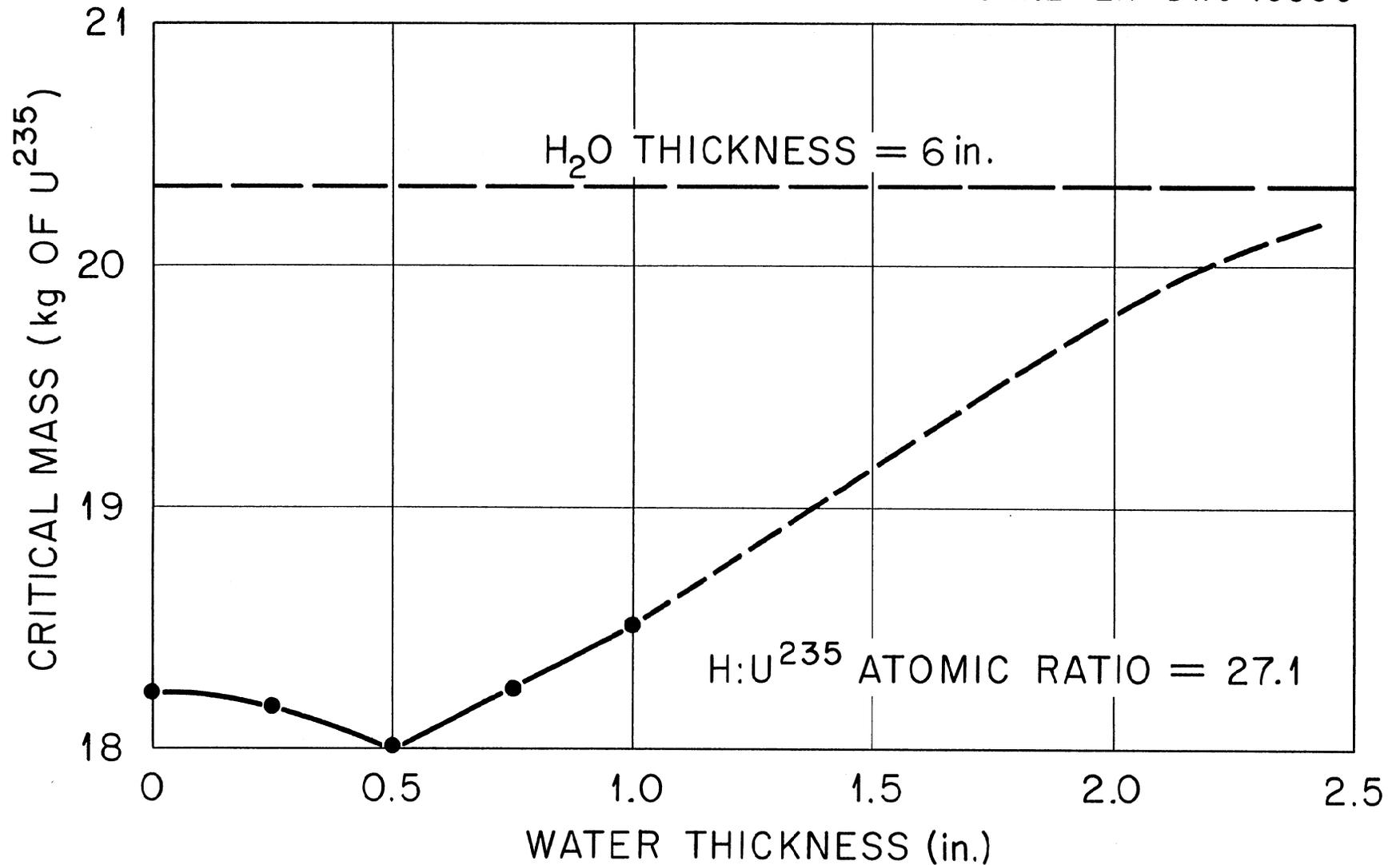
Fig. 23. Critical Mass as a Function of the Thickness of Water Between the Bottom of a 20-in.-dia Cylinder Containing an Enriched U<sup>235</sup> Solution and a 5.5-in.-thick Carbon Reflector.
