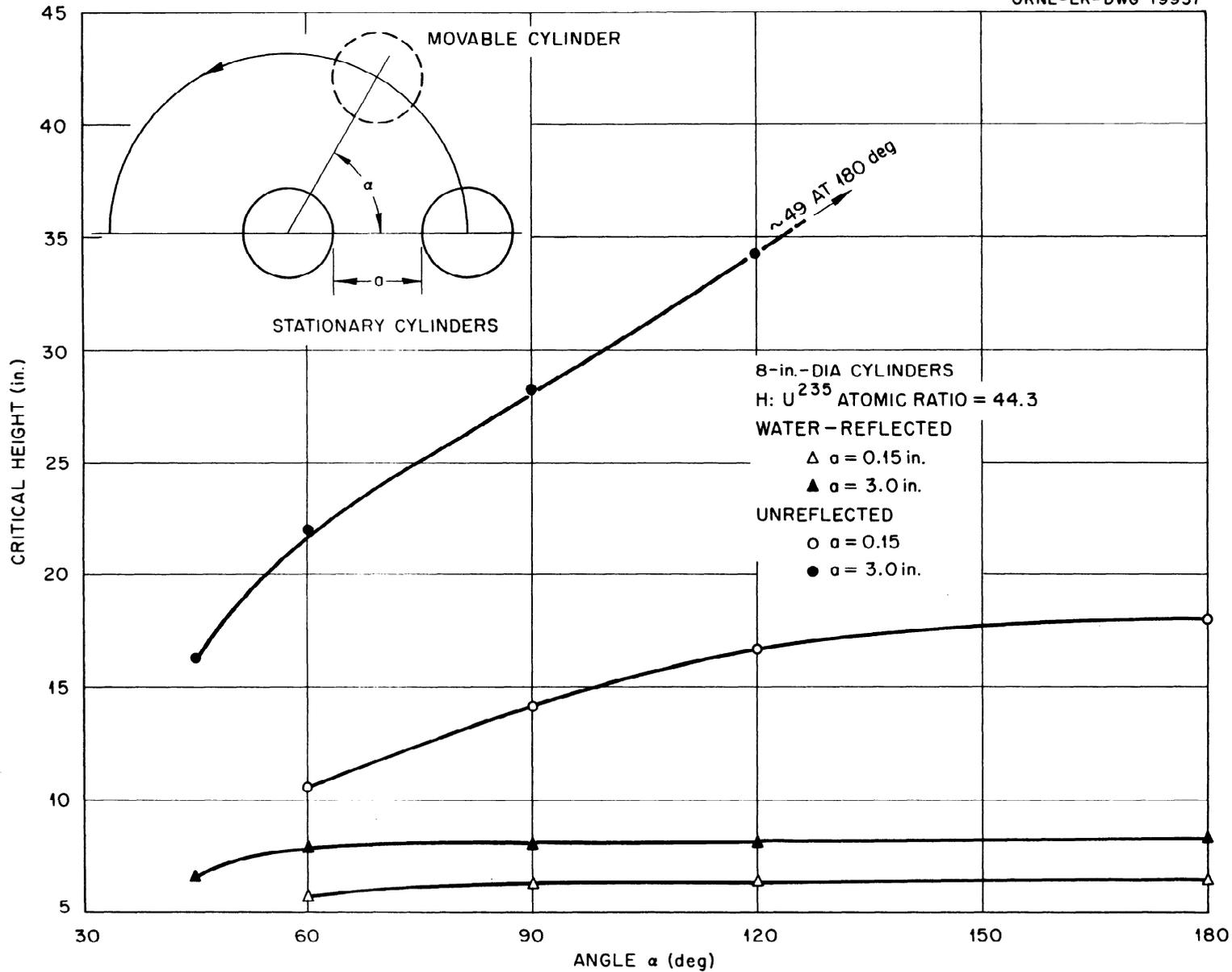
Fig. 9. Critical Height of Three Unreflected and Water-Reflected 8-in.-dia Aluminum Cylinders Containing an Enriched  $U^{235}$  Solution as a Function of the Vertex Angle of an Isosceles Triangle Describing the Relative Locations of the Cylinders.
