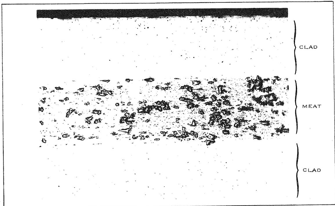
Fig. H-3 Photomicrograph of transverse-type specimen from the rupture area of plate D-2321 (50x).
