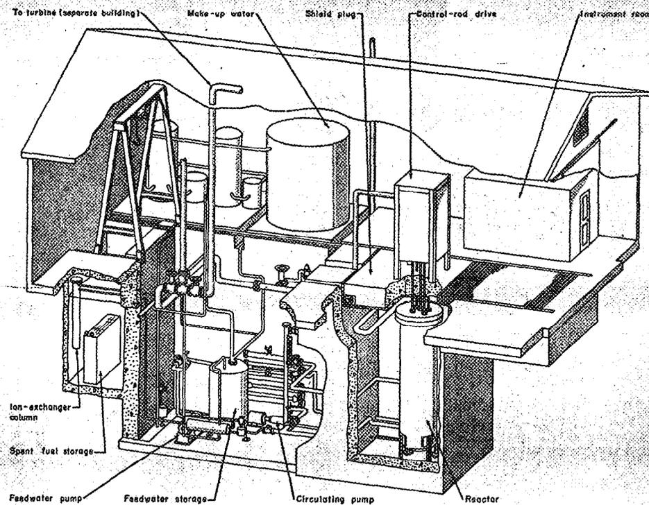
FIG. 2. US's 15-Mw prototype boiling-water power reactor (Borax-3) plant
