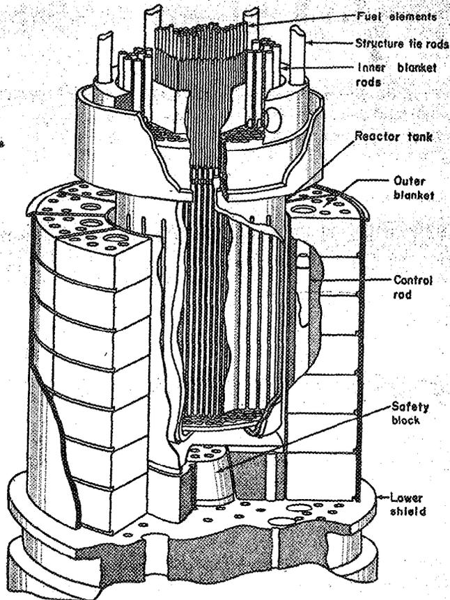
FIG. 15. EBR-1 cutaway
