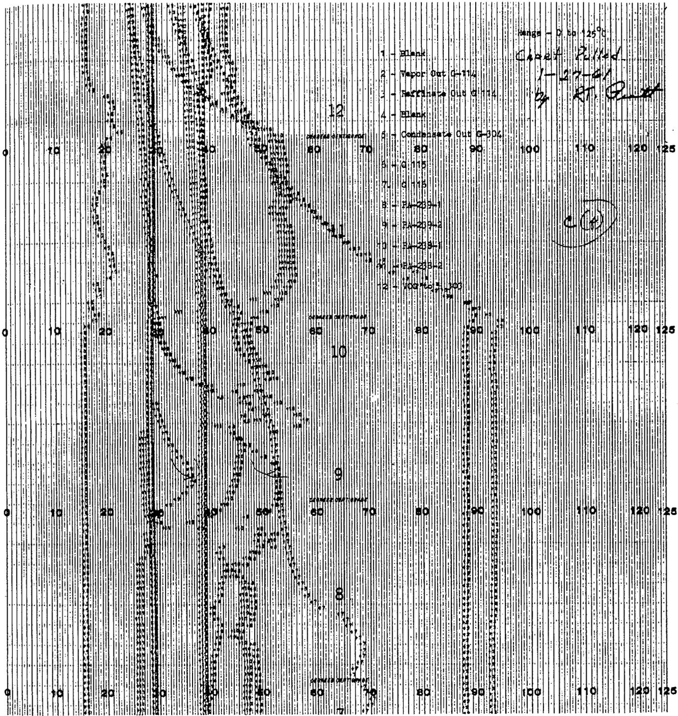
TEMPERATURE OF DISCHARGE LINE-PUMPS PA-238 - PA-239
