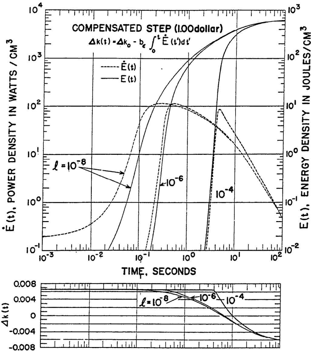
Fig. 8. Energy model computation of power versus time for an initial reactivity of 1.0 dollar above delayed critical for three different neutron lifetime values,  $l = 10^{-8}$ ,  $10^{-6}$ , and  $10^{-4}$  sec. Below are the corresponding curves of reactivity versus time.
