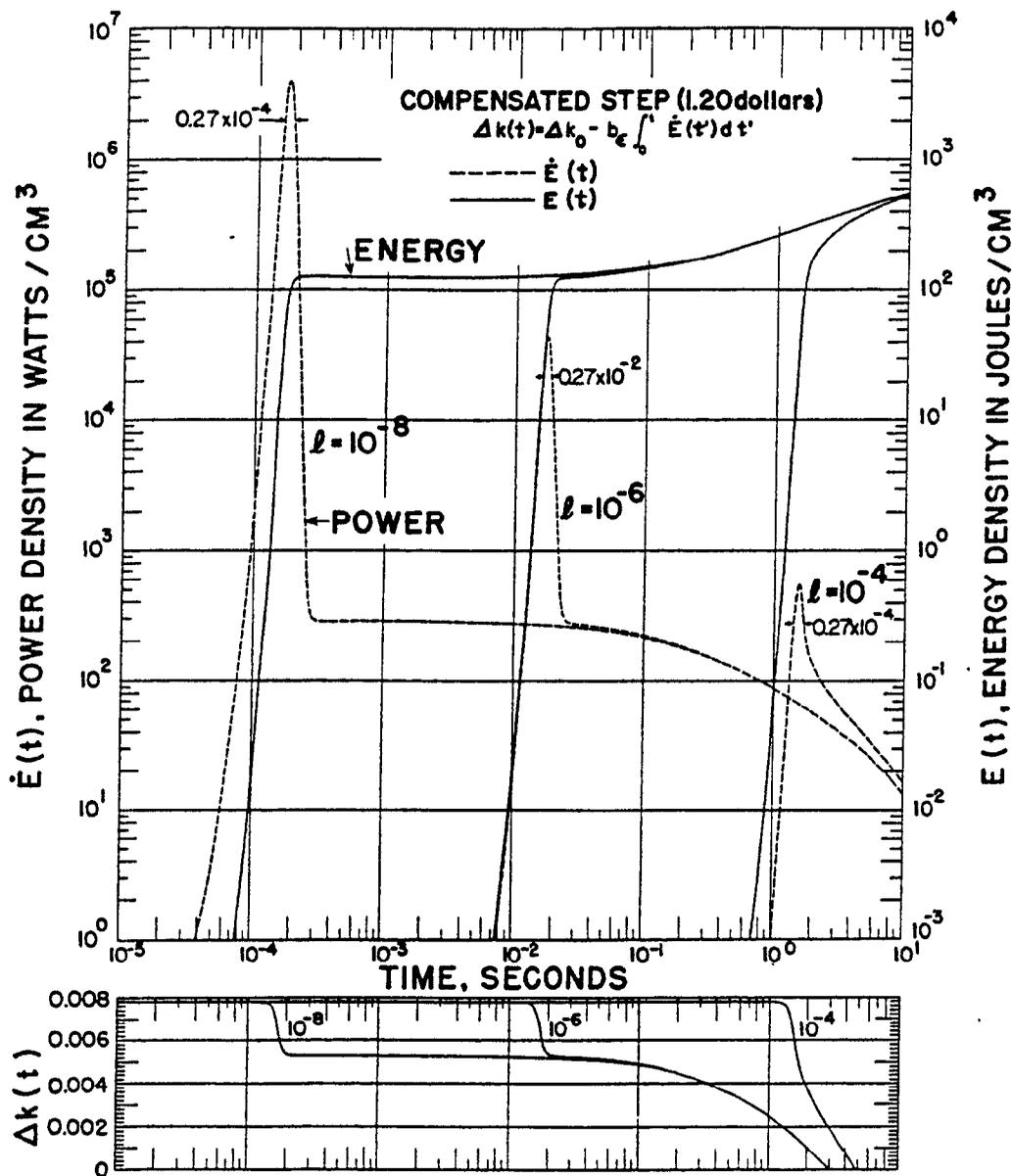
Fig. 7. Energy model computation of power versus time and energy release versus time, for an initial reactivity of 1.2 dollars above delayed critical for three different neutron lifetime values,  $\lambda = 10^{-8}$ ,  $10^{-6}$ , and  $10^{-4}$  sec. Below are the corresponding curves of reactivity versus time.
