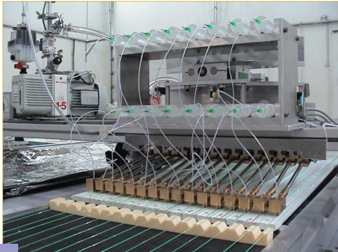
**Opera fiber gluing system**
