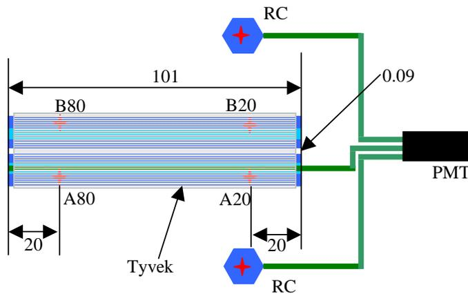
Fig. 2. Schematic of the set-up used for strip measurements. (All dimensions are given in cm). The letters RC denote the reference cells.
