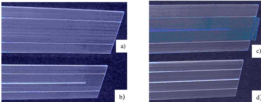
Fig. 1. a) A strip after extrusion; b) The same strip with a machined separation groove; c) The strip with blue tape; d) The trimmed strip with the glued separation groove.
