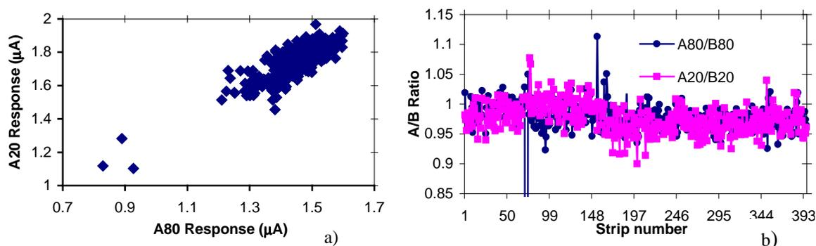
Fig. 5. a) A20 response versus A80 (for all strips) illustrates the uniformity at A20 and at A80 for all strips; b) Asymmetry across the strip (the strip number is not associated with production time).
