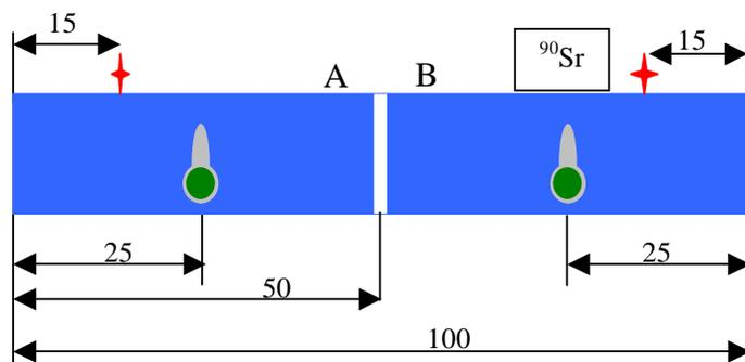
Fig. 3. A schematic used for a strip orientation and a radioactive source positioning (dimensions are given in mm).
