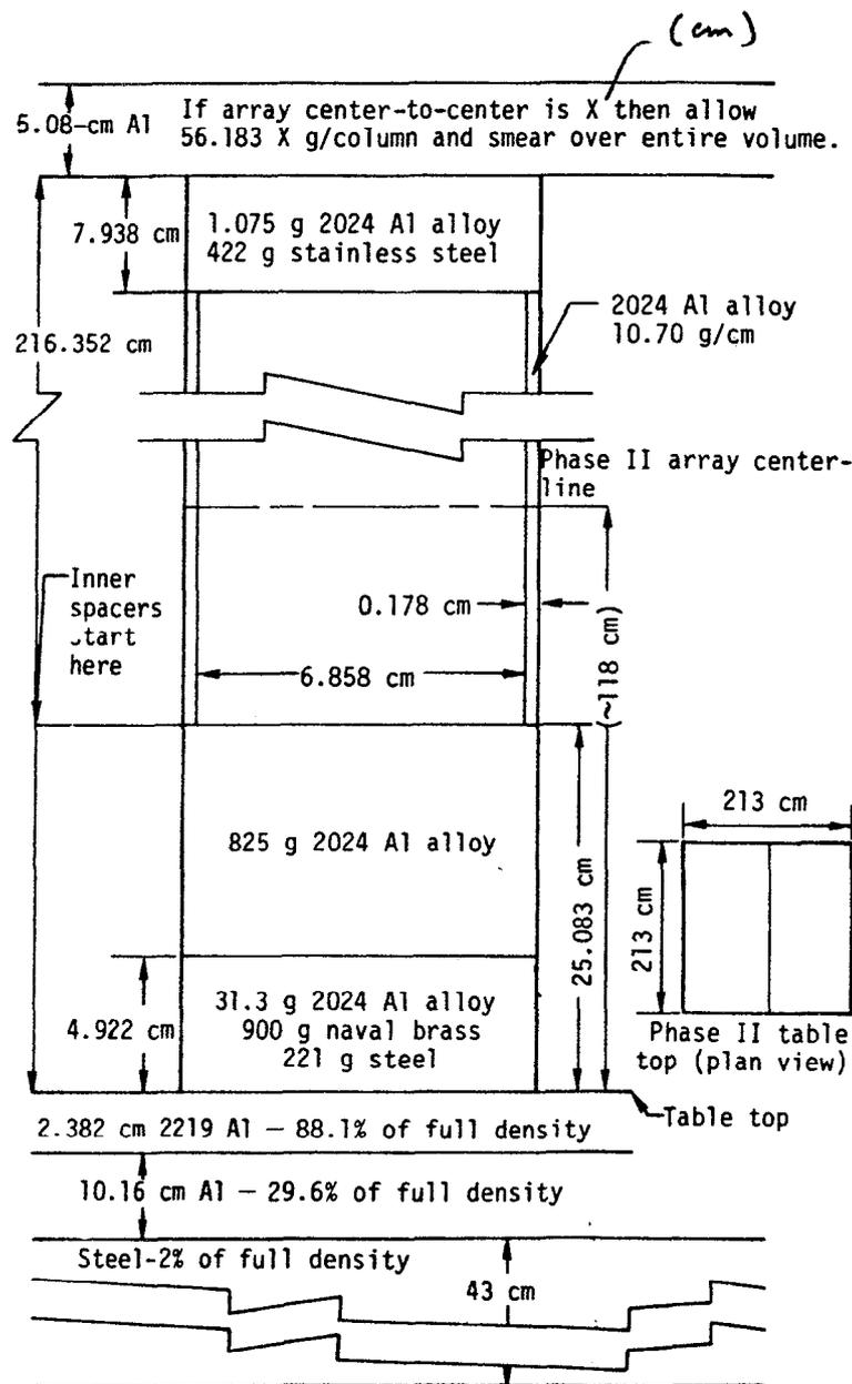
Fig. 6. Schematic drawing of Phase II support apparatus.
