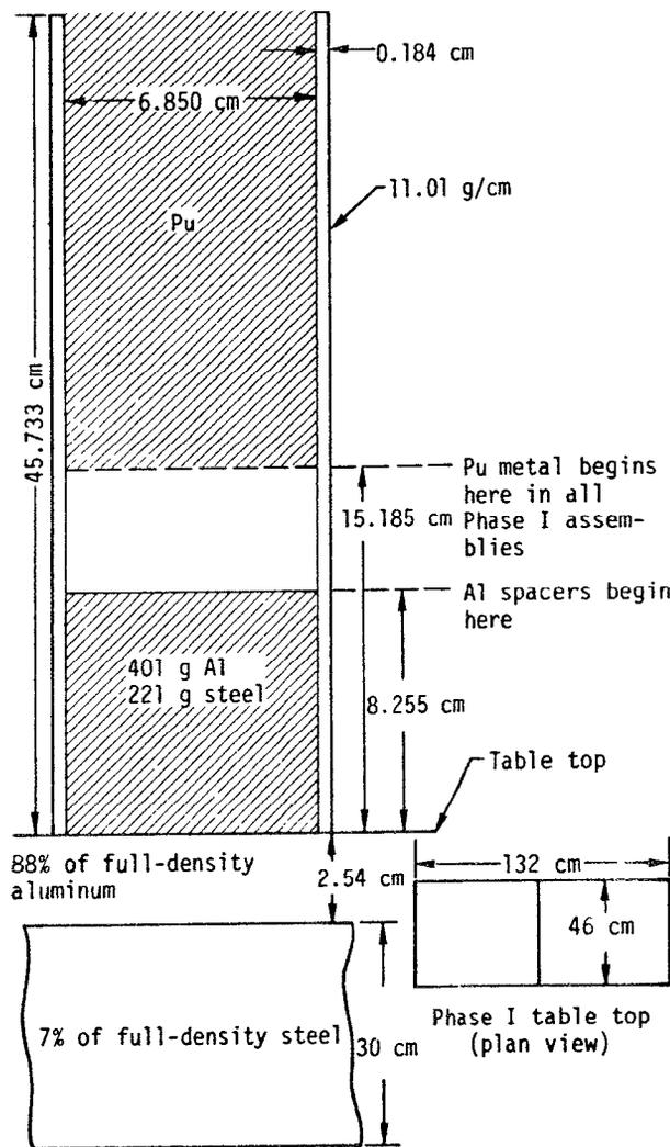
Fig. 4. Schematic drawing of Phase I support apparatus.
