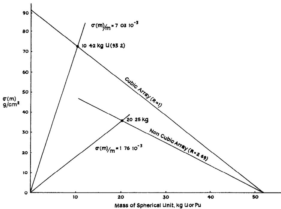
3 Mixed Oxide cubic array calculations in the  $\sigma(m), m$  plane.
