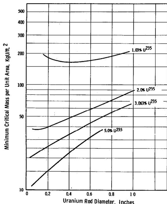
Fig. 15. Estimated minimum critical mass per unit area for 1, 2, 3, and 5 wt. % U-235 enriched uranium rods for water as a function of rod diameter.
