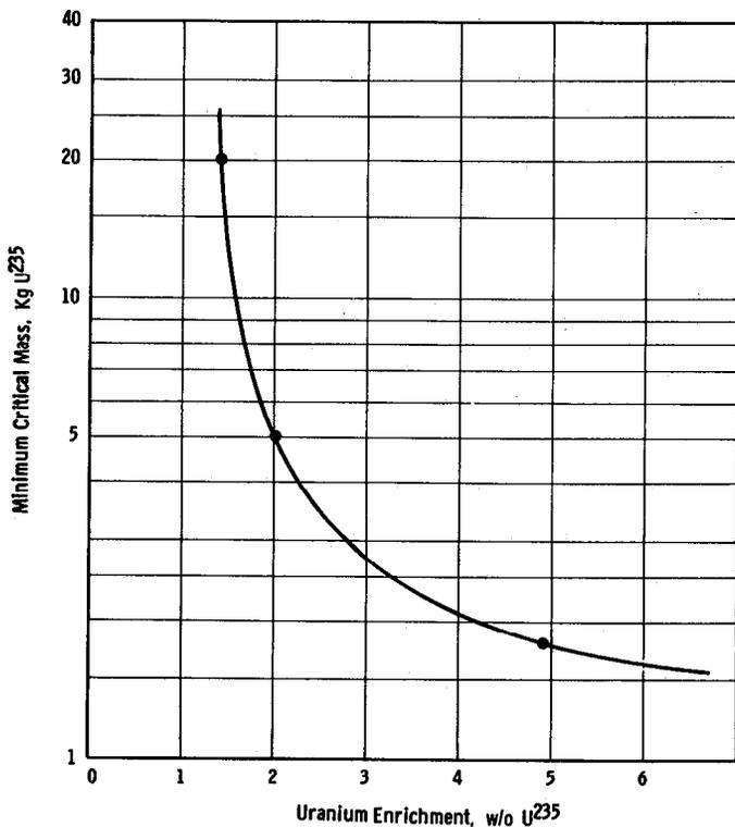
Fig. 3. Minimum critical mass for uranium solution as a function of U-235 enrichment (spherical geometry-water reflected).
