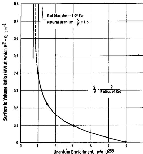
Fig. 14. Estimated surface-to-volume ratios of large rods (billets) which result in zero bucklings and infinite critical mass as a function of U-235 enrichment.
