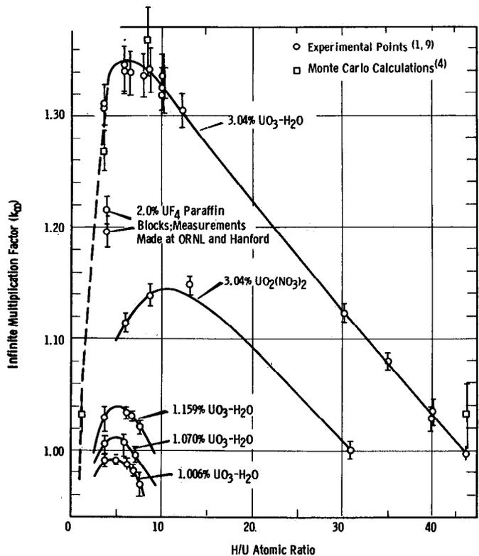
Fig. 4.  $k_{\infty}$  for  $UO_3$ -water and uranyl nitrate systems as a function of hydrogen-uranium atomic ratio.
