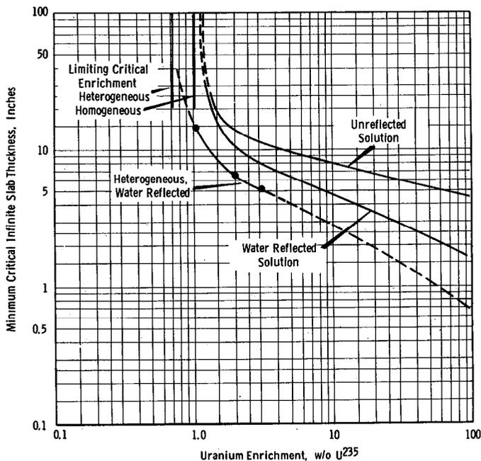
Fig. 12. Minimum critical slab thickness for heterogeneous and homogeneous uranium-water systems as a function of U-235 enrichment.
