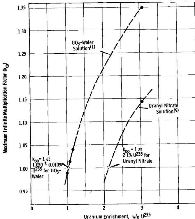
Fig. 5. Maximum  $k_{\infty}$  for  $\text{UO}_3$ -water and uranyl nitrate systems as a function U-235 enrichment.
