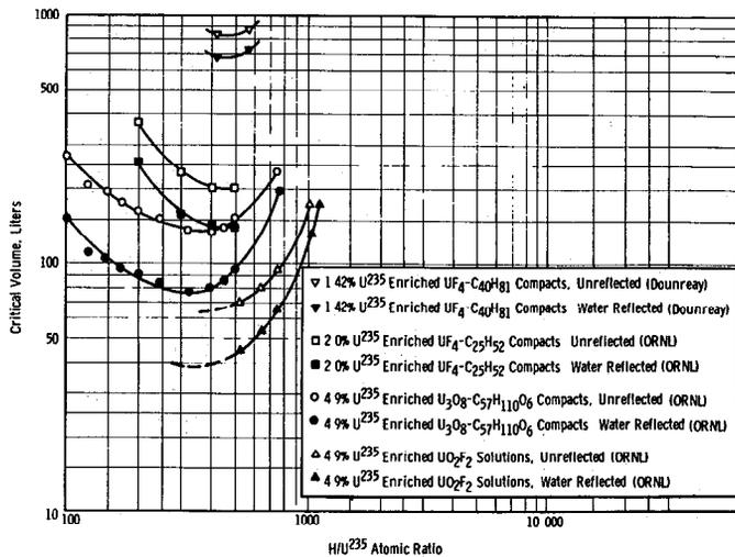
Fig. 2. Critical volume of U-235 enriched uranium in spherical geometry as a function of hydrogen-U-235 ratio as determined from experimental measurements
