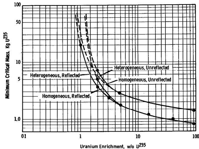
Fig. 9. Minimum critical mass for heterogeneous and homogeneous uranium-water systems as a function of U-235 enrichment.
