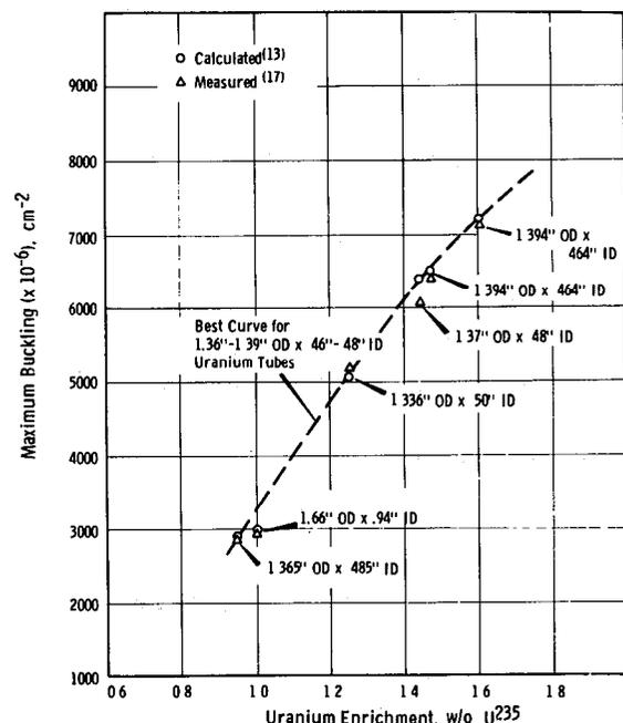
Fig. 13. Measured and calculated maximum material bucklings for uranium tubes in water as a function of U-235 enrichment.
