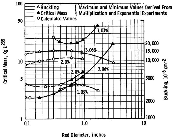
Fig. 8. Minimum water reflected critical mass and maximum buckling for lattices of 1.03, 2.0, and 3.06 wt. % U-235 enriched uranium rods in water as a function of rod diameter.
