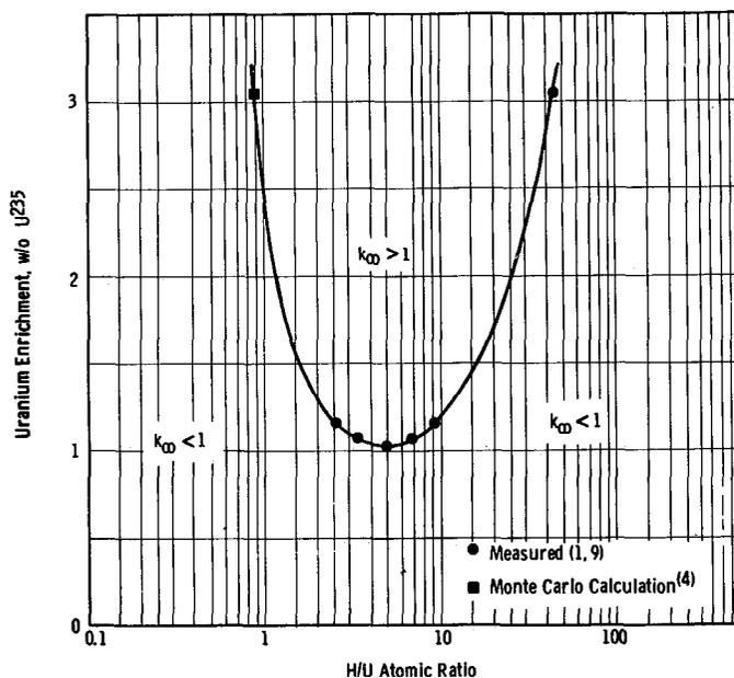
Fig. 6. Hydrogen-uranium atomic ratios at which  $k_{\infty} = 1$  for  $\text{UO}_3$ -water systems as a function of U-235 enrichment.
