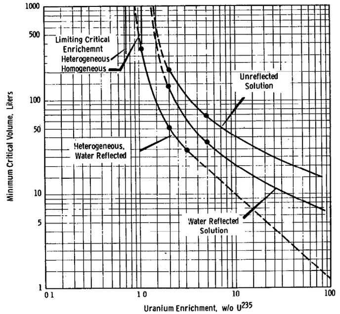
Fig. 10. Minimum critical volume for heterogeneous and homogeneous uranium-water systems as a function of U-235 enrichment.
