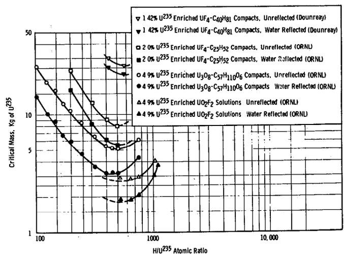
Fig. 1. Critical mass of U-235 enriched uranium in spherical geometry as a function of hydrogen-U-235 atomic ratio as determined from experimental measurements.
