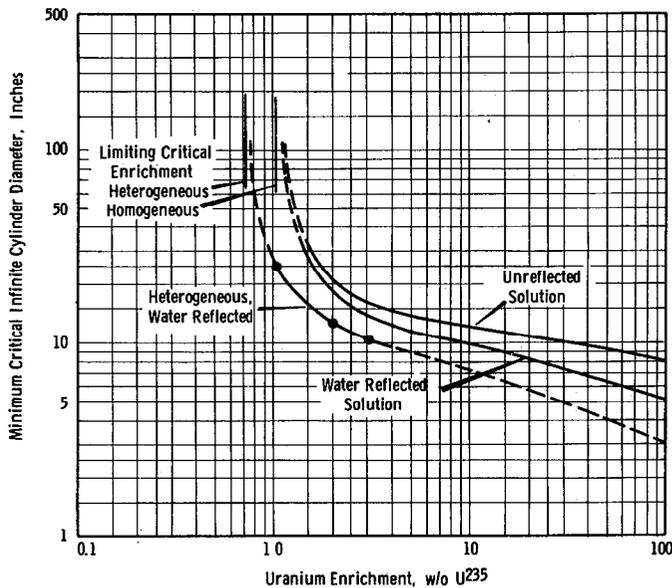
Fig. 11. Minimum critical cylinder diameter for heterogeneous and homogeneous uranium-water systems as a function of U-235 enrichment.
