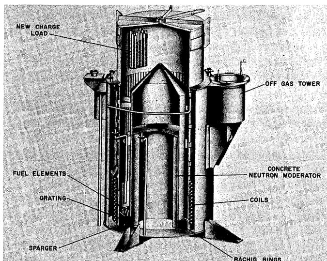
Fig. 16. Annular dissolver.
