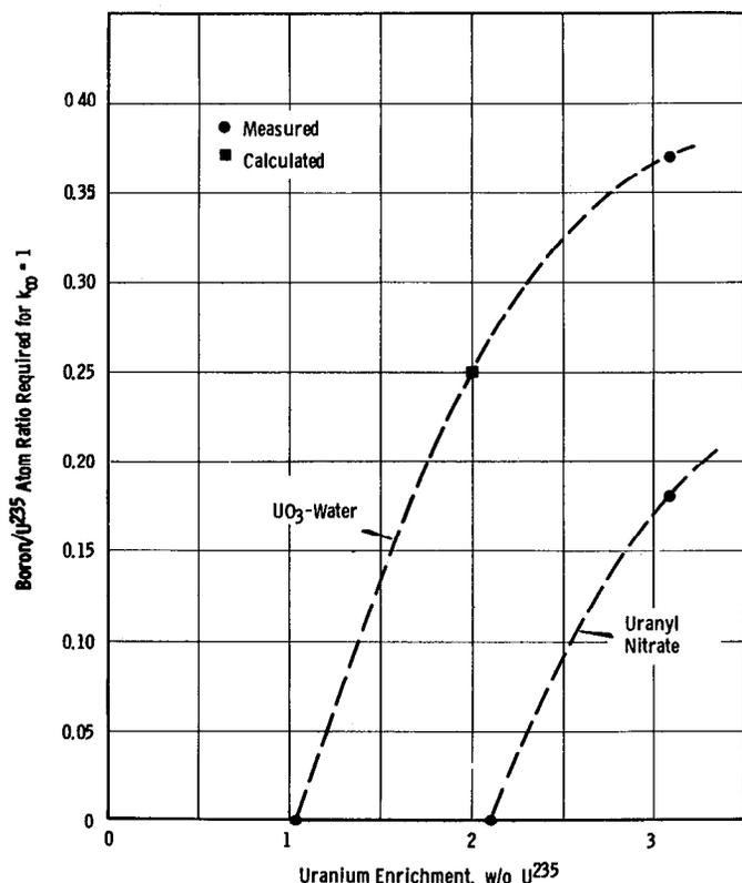
Fig. 7. Estimated amount of boron required in  $\text{UO}_3$ -water and uranyl nitrate systems to reduce  $k_\infty$  to unity as a function of U-235 enrichment.
