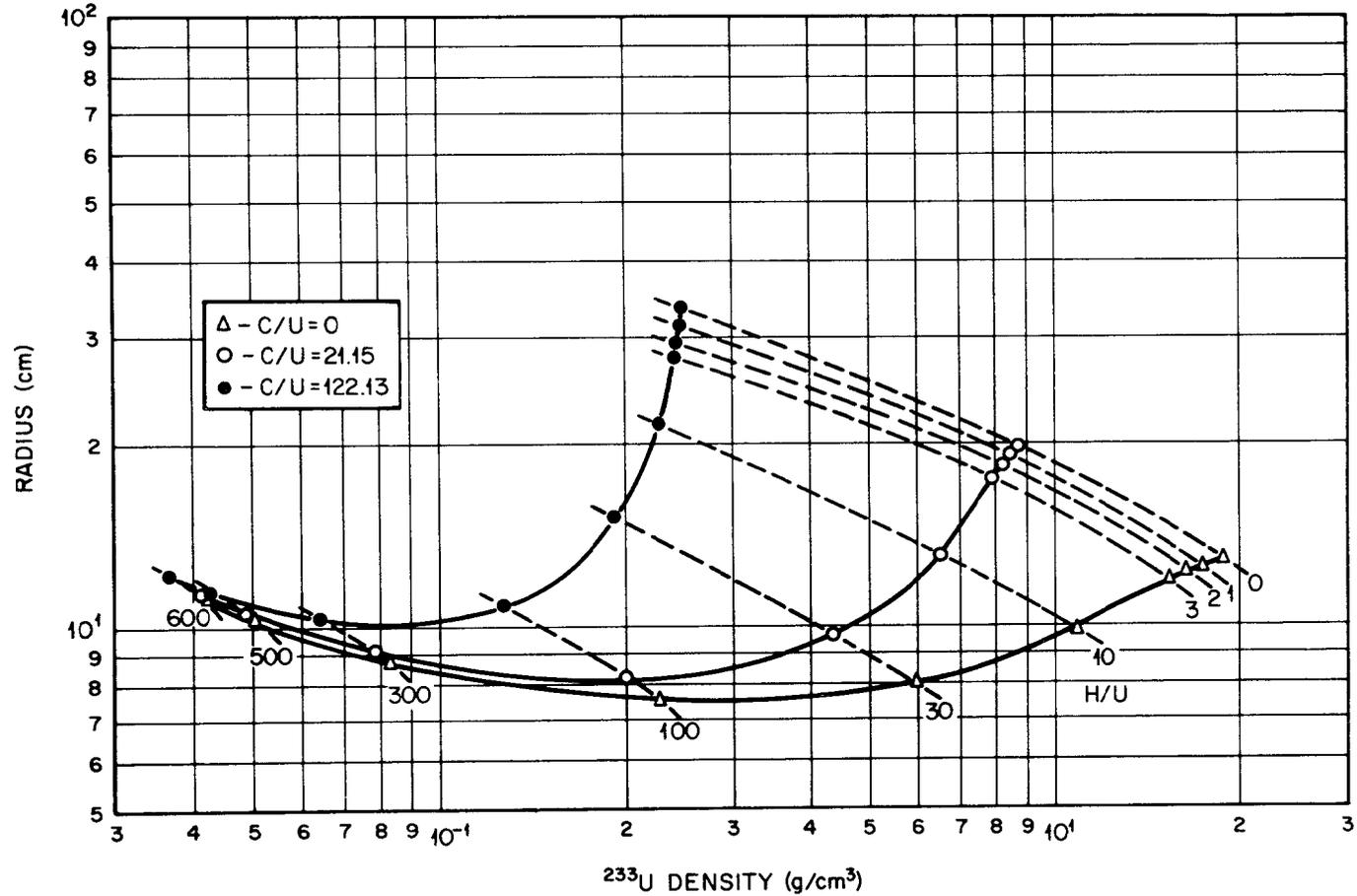
Fig. 6. Estimated Critical Radius of Infinite Cylinders of Water-Moderated  $(\text{Th,U})\text{O}_2$  (water reflected) with Various C/U-Th:U = 4:1.
