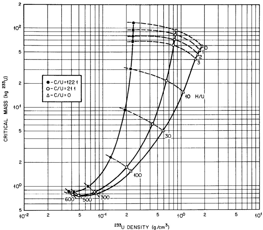
Fig. 3. Critical Masses of (4 Th:1 <sup>233</sup>U)O<sub>2</sub> in Spherical Geometry (water reflected) with Various H/U and C/U.
