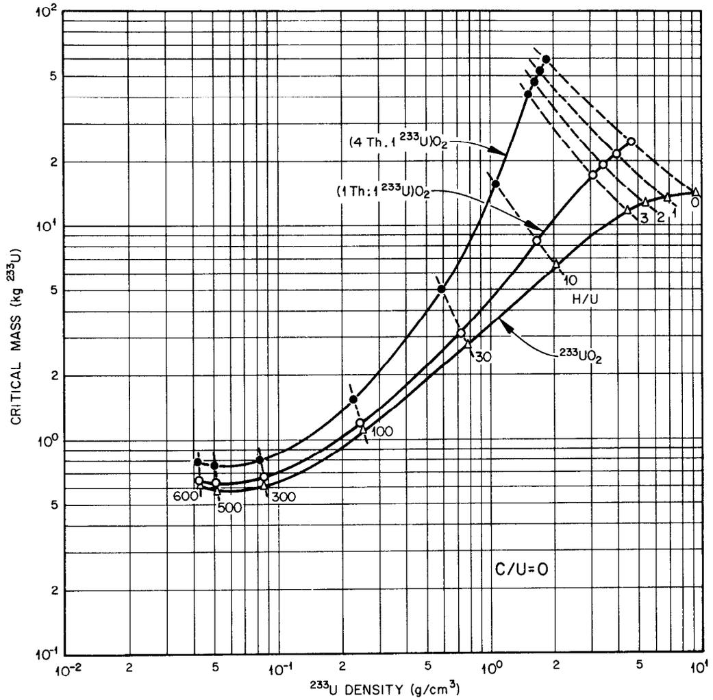
Fig. 7. Critical Masses of  $^{233}\text{UO}_2$  in Spherical Geometry with Various Amounts of  $\text{ThO}_2$  (water reflected).
