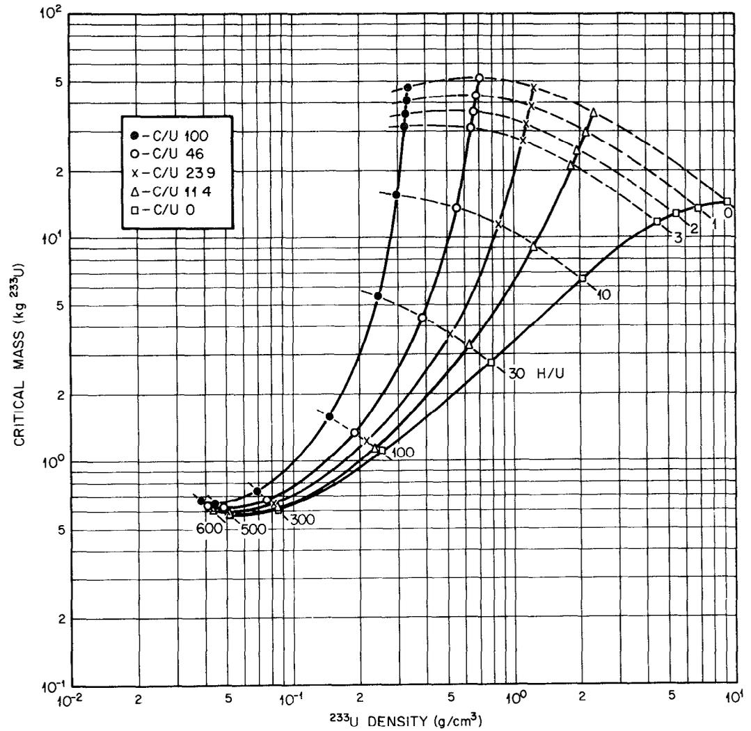
Fig. 1. Critical Masses of  $^{233}\text{UO}_2$  in Spherical Geometry (water reflected) with Various H/U and C/U.
