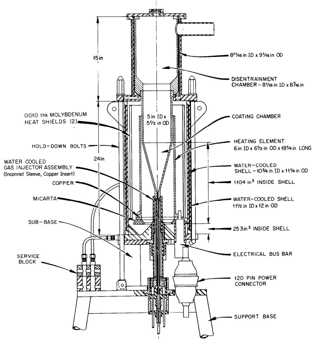
Fig. 9. Coater for HTGR Recycle Fuel
