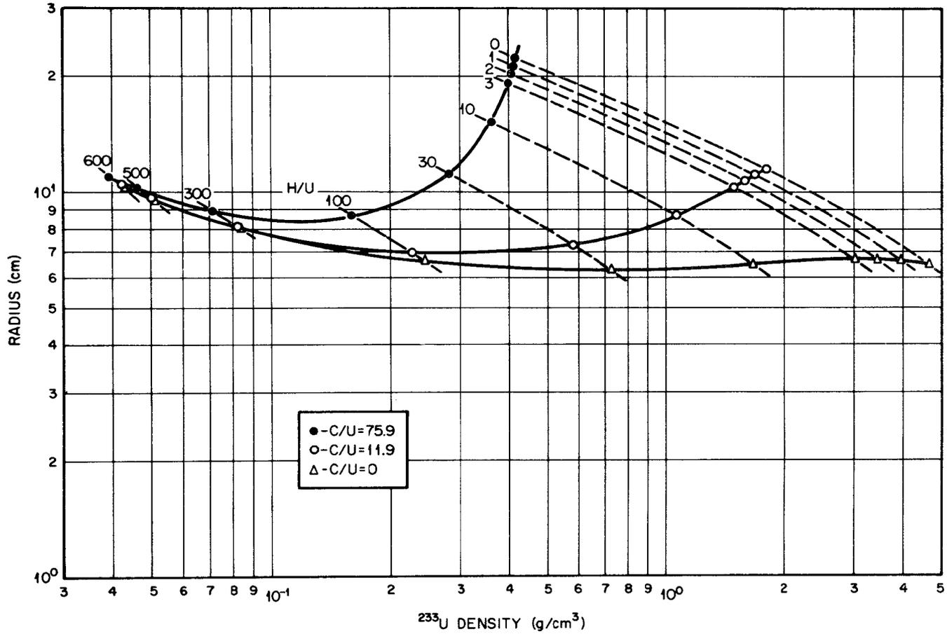
Fig. 5. Estimated Critical Radius of Infinite Cylinders of Water-Moderated  $(\text{Th}, \text{U})\text{O}_2$  (water reflected) with Various C/U-Th:U = 1:1.
