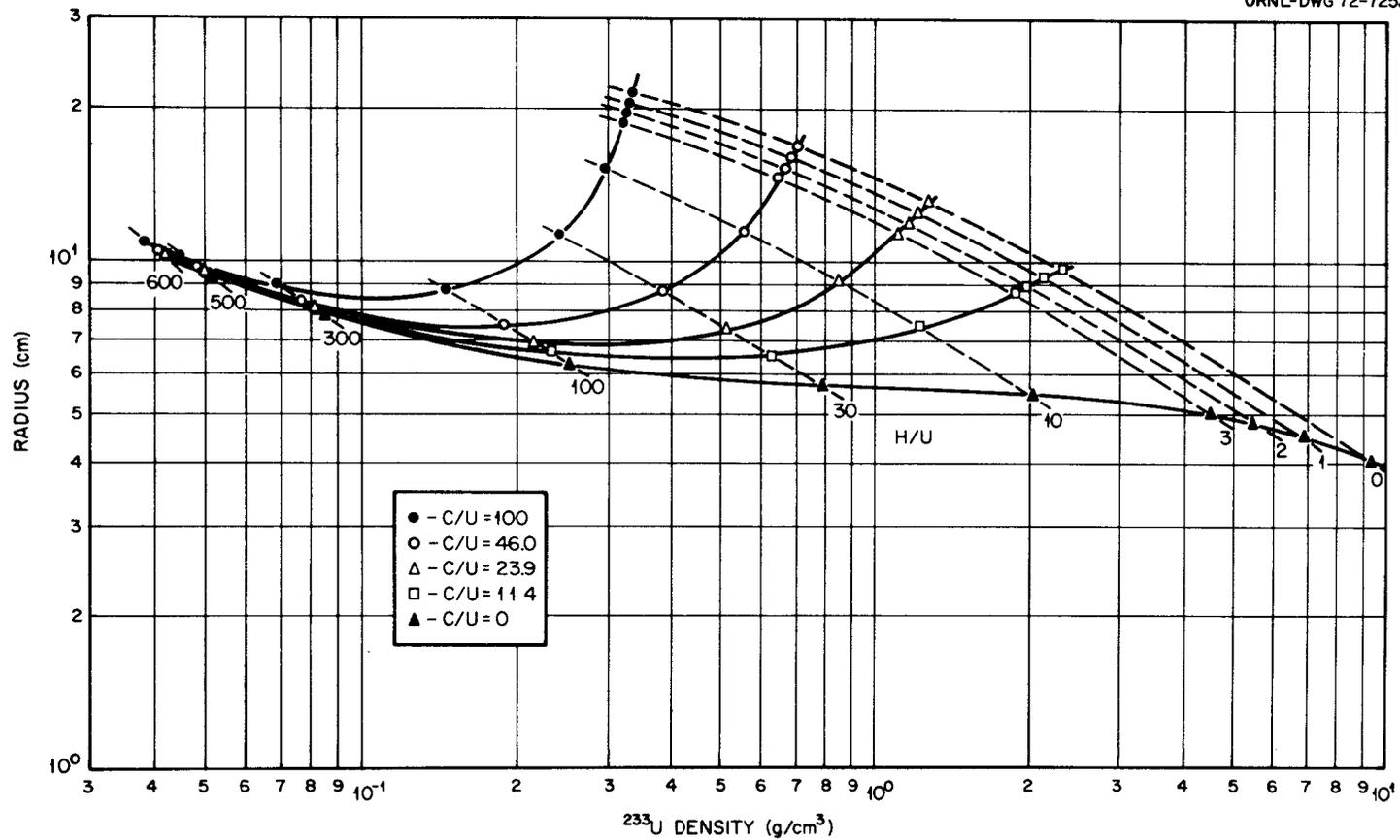
Fig. 4. Estimated Critical Radius of Infinite Cylinders of Water-Moderated  $(\text{Th},\text{U})\text{O}_2$  (water reflected) with Various C/U-Th:U = 0:1.
