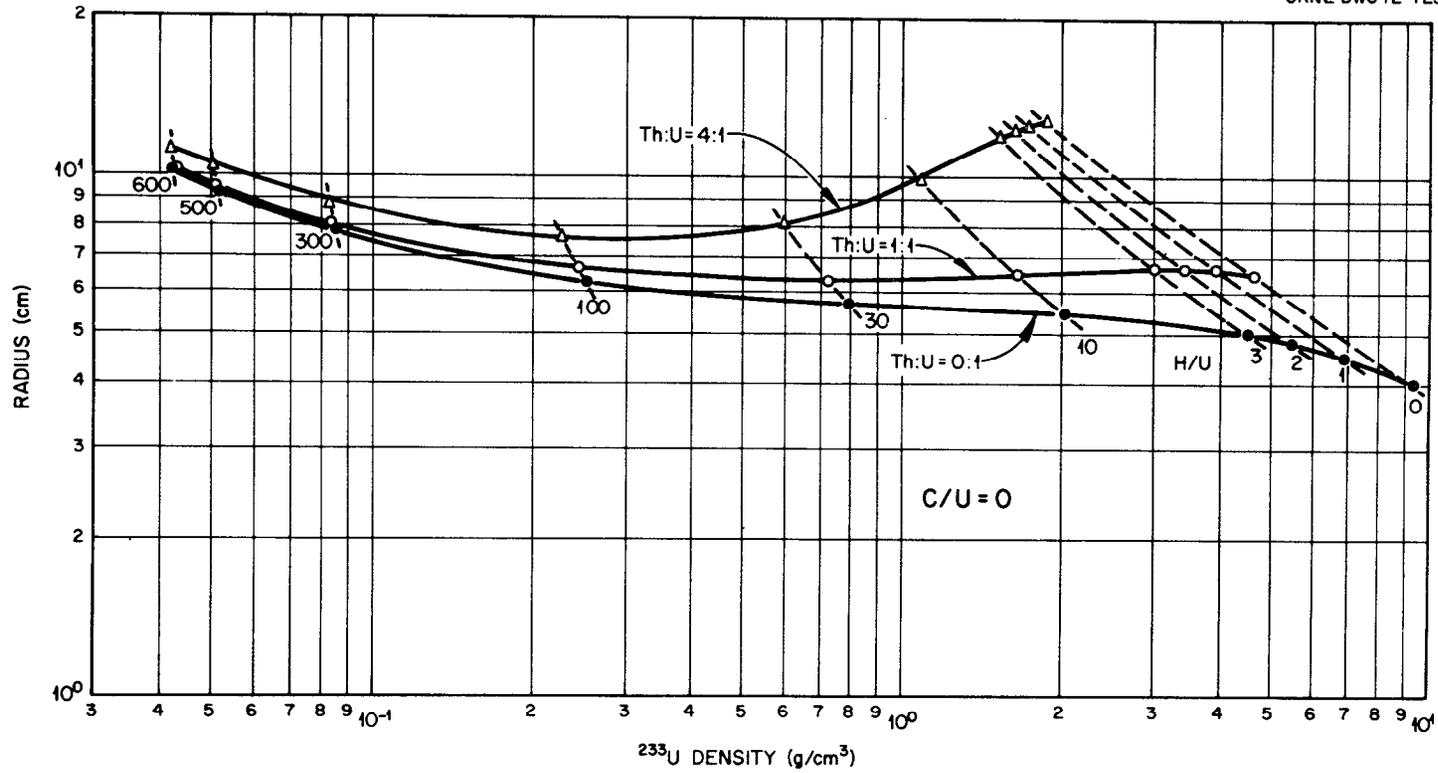
Fig. 8. Calculated Critical Radius of Infinite Cylinders of Water-Moderated  $^{233}\text{UO}_2$  (water reflected) with Various Amounts of  $\text{ThO}_2$ .
