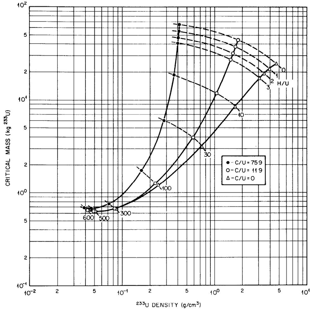
Fig. 2. Critical Masses of  $(1 \text{ Th}:1 \text{ }^{233}\text{U})\text{O}_2$  in Spherical Geometry (water reflected) with Various  $\text{H}/\text{U}$  and  $\text{C}/\text{U}$ .
