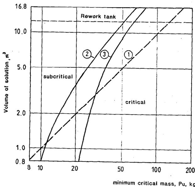
Figure 5: Condition for criticality in the rework tank
