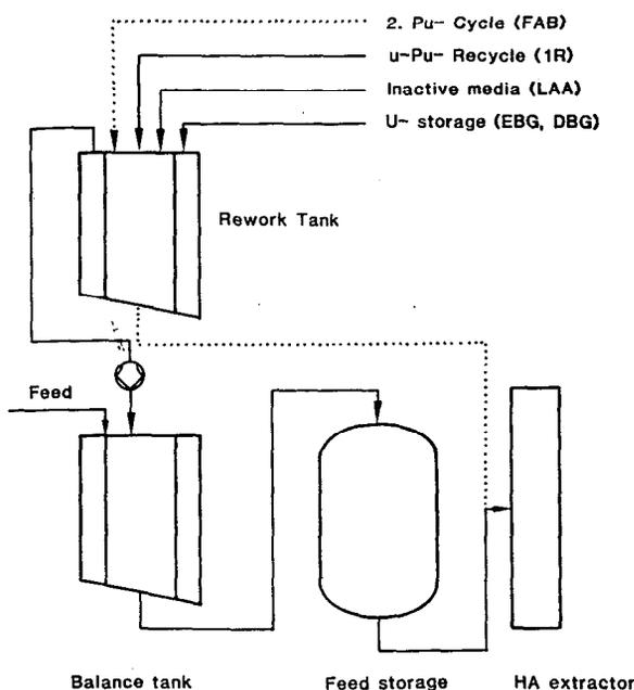
Figure 2: Principal arrangement of feed storage and rework tank
