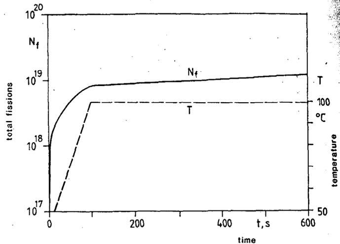
Figure 1: Total fissions and temperature for a criticality excursion in a solution
