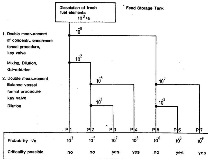
Figure 4: Probabilities for a criticality in the feed storage tank as a result of dissolution of fresh fuel elements.
