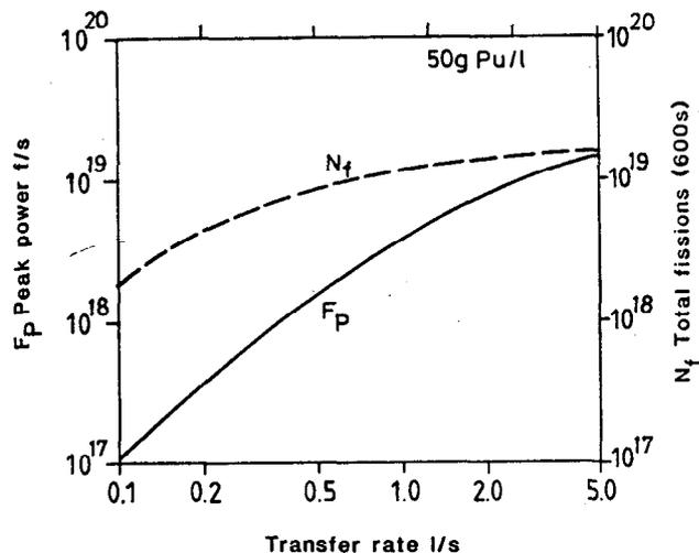
Figure 6: Variation of pump capacity for accidental transfer of plutonium solution
