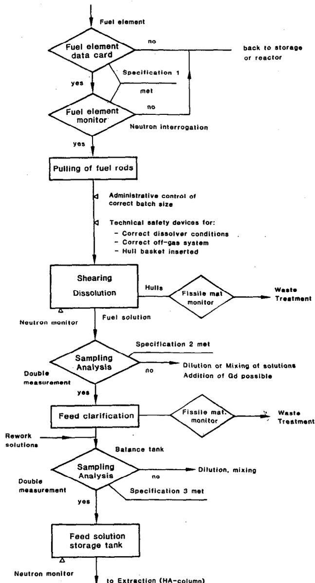
**Figure 3:** Control of parameters relevant for criticality safety in headend and feed clarification
