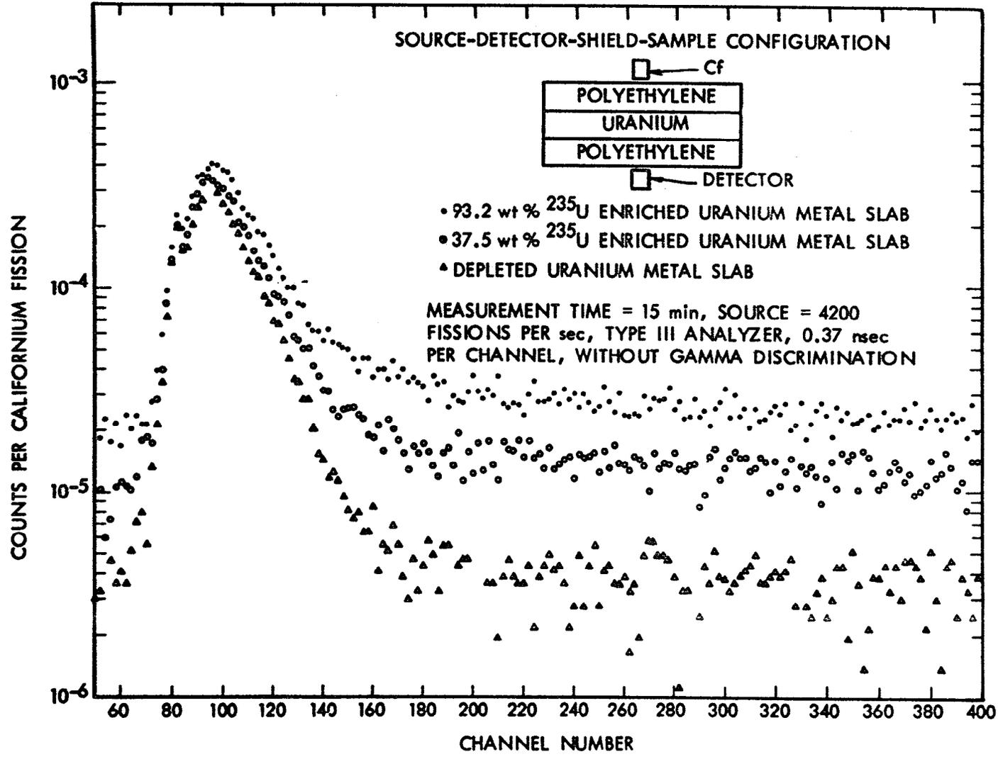
Fig. 8. Counts vs Time with the Source and Detector on Opposite Sides of the Sample and with a 1-in.-thick Polyethylene Shield.
