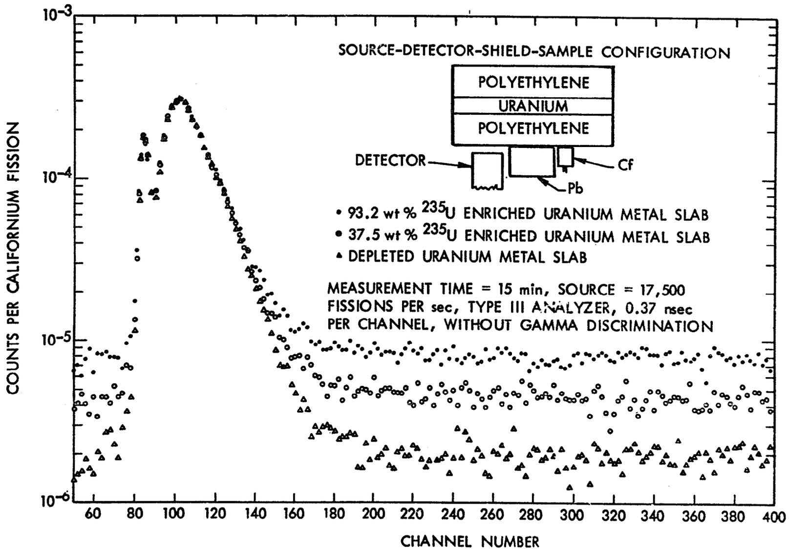
Fig. 11. Counts vs Time with the Source and Detector on the Same Side of the Sample and with a 2-in.-thick Polyethylene Shield.
