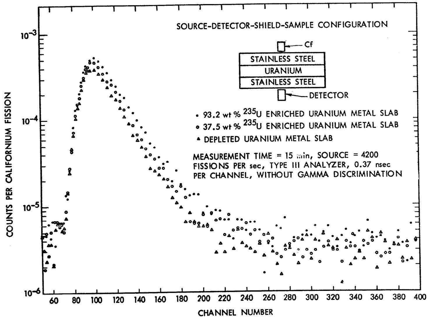
Fig. 12. Counts vs Time with the Source and Detector on Opposite Sides of the Sample and with a 1-in.-thick Stainless Steel Shield.
