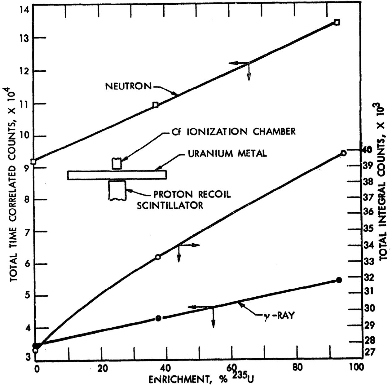
Fig. 6. Total Time Correlated Counts from a Randomly Pulsed Neutron Measurement with Californium and Total Integral Counts from a Source Neutron Multiplication Measurement as a Function of  $^{235}\text{U}$  Enrichment of Unshielded Samples with the Source and Detector on Opposite Sides.
