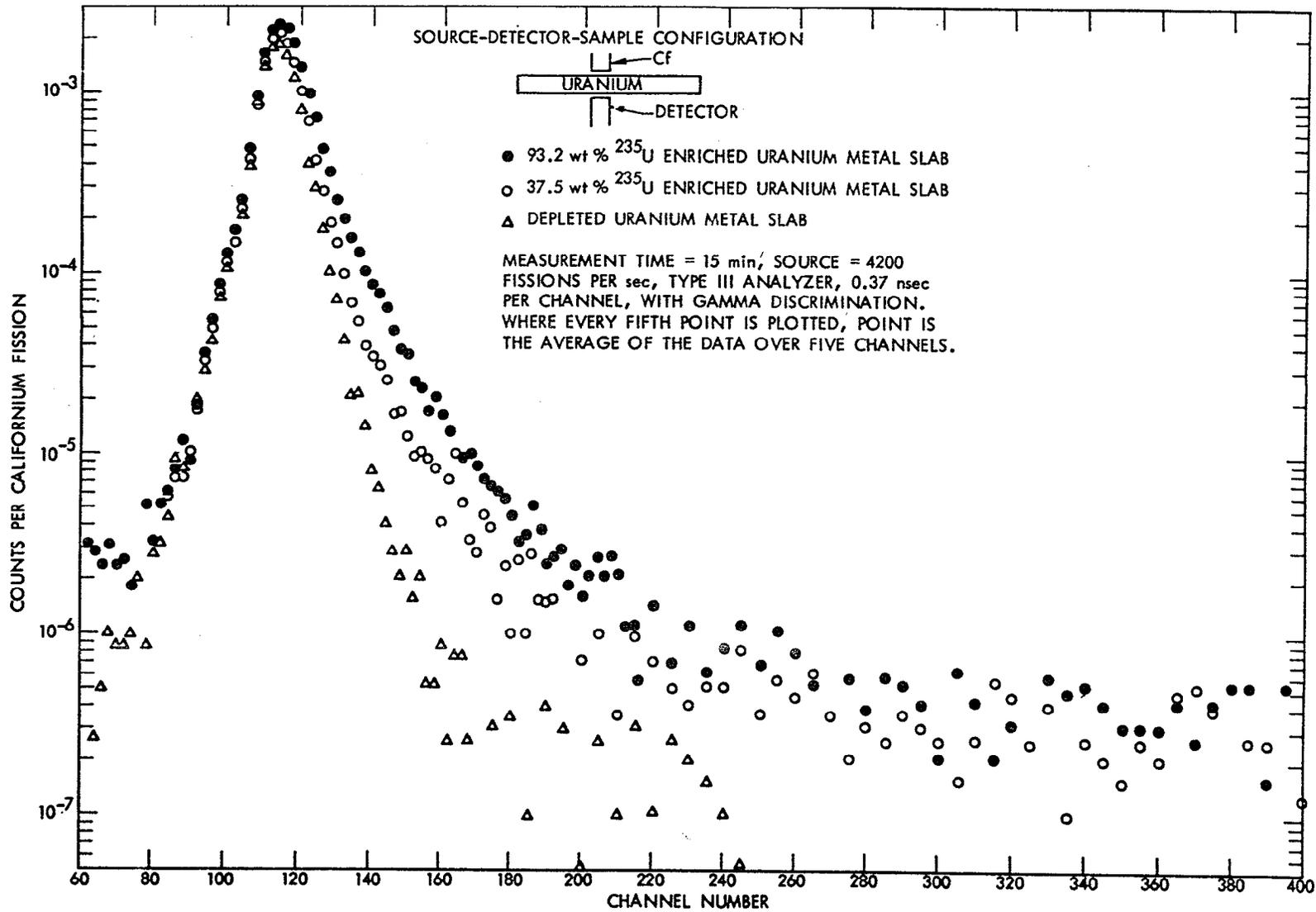
Fig. 4. Neutron Counts vs Time with the Source and Detector on Opposite Sides of the Unshielded Samples.
