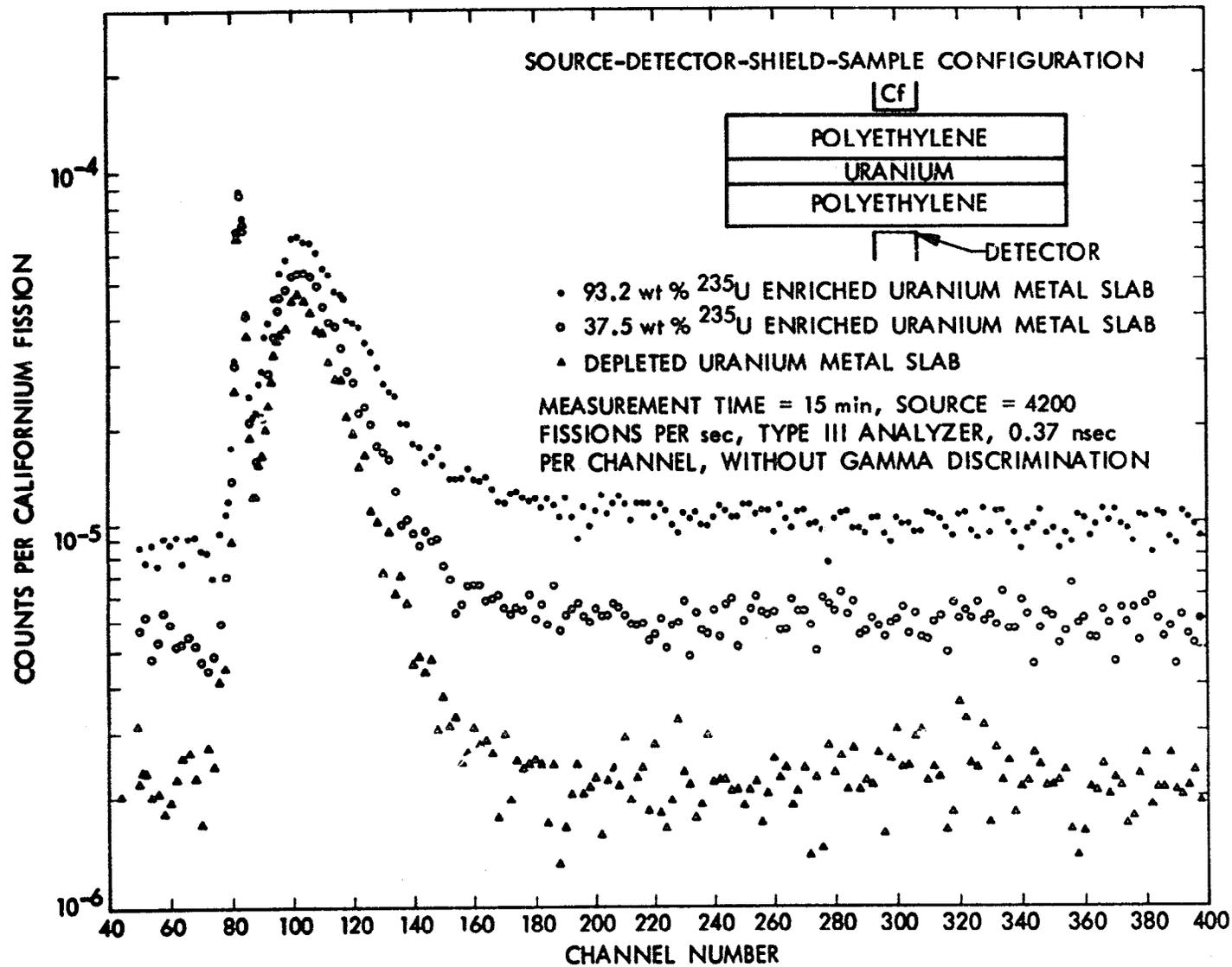
Fig. 10. Counts vs Time with the Source and Detector on the Same Side of the Sample and with a 1-in.-thick Polyethylene Shield.
