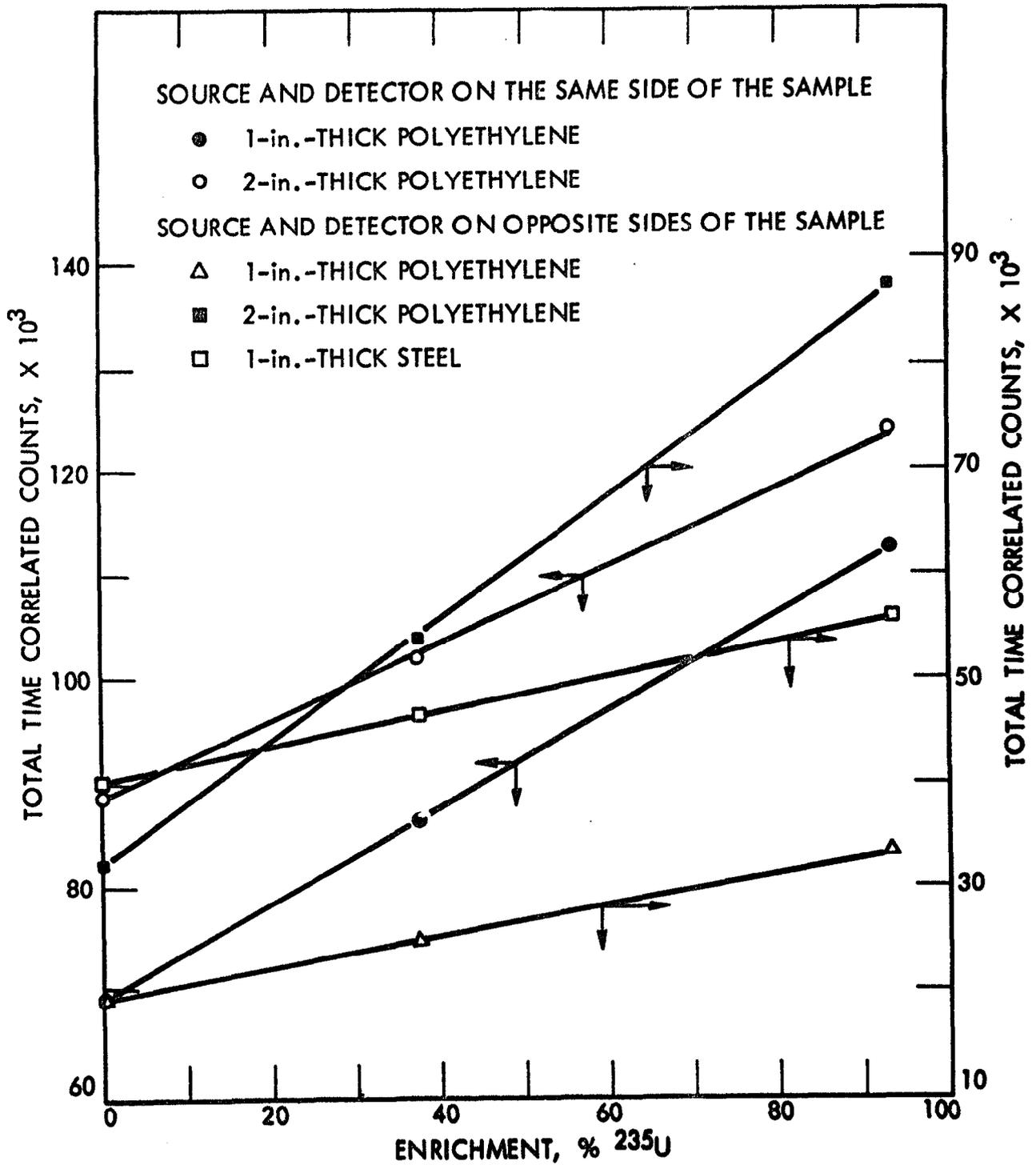
Fig. 14. Total Time Correlated Counts as a Function of  $^{235}\text{U}$  Enrichment for Various Source-Detector-Shield Configurations.
