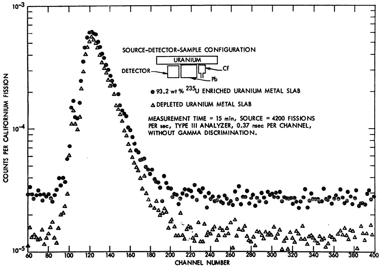
Fig. 7. Counts vs Time with the Source and Detector on the Same Side of Unshielded Samples.
