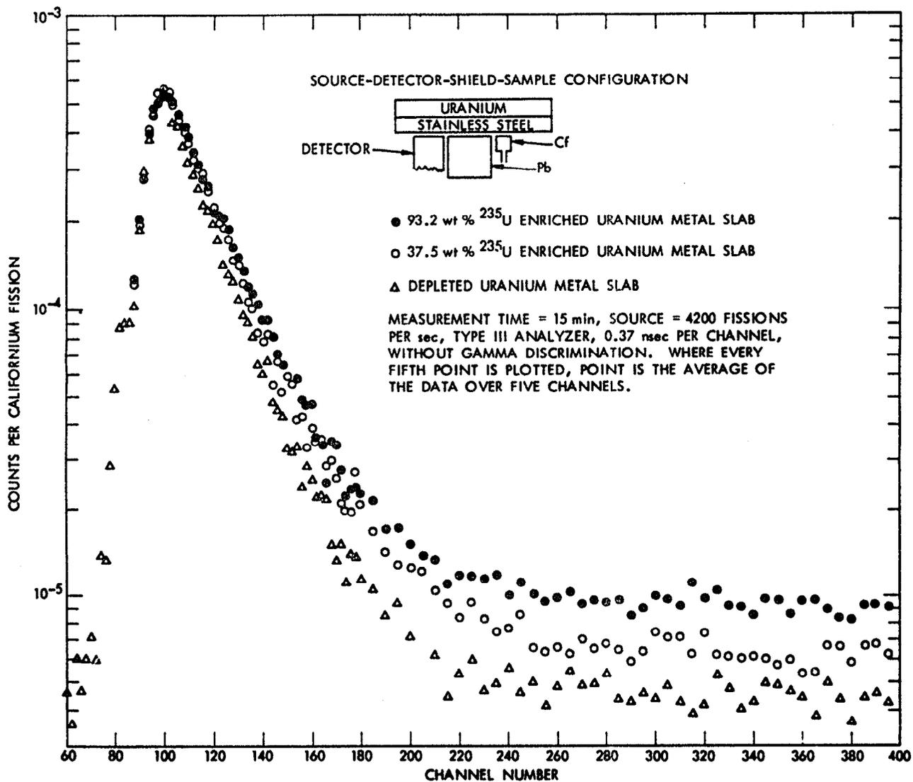
Fig. 13. Counts vs Time with the Source and Detector on the Same Side of the Sample and with a 1-in.-thick Stainless Steel Shield.
