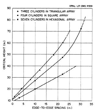
Fig. 3.7.3. Critical Solution Height as a Function of Edge-to-Edge Spacing of Unreflected Triangular, Hexagonal, and Square Arrays of 9.5-in.-dia Aluminum Cylinders Containing Aqueous Solutions of 93.2% U<sup>235</sup>-Enriched Uranyl Fluoride (H:U<sup>235</sup> Atomic Ratio = 297).
