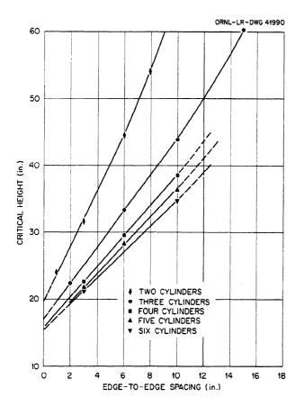
Fig. 3.7.2. Critical Solution Height as a Function of Edge-to-Edge Spacing of Unreflected Straight-Line Arrays of 9.5-in.-dia Aluminum Cylinders Containing Aqueous Solutions of 93.2% U<sup>235</sup>-Enriched Uranyl Fluoride (H:U<sup>235</sup> Atomic Ratio = 297).
