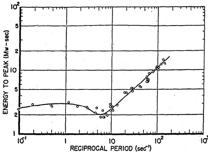
FIG. 13. Energy released to the time of maximum reactor power as a function of reciprocal reactor period.
