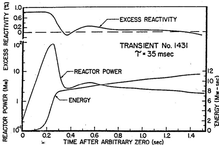
FIG. 19. Instantaneous excess reactivity during a 35-msec period transient test. Also shown are reactor power and energy release.
