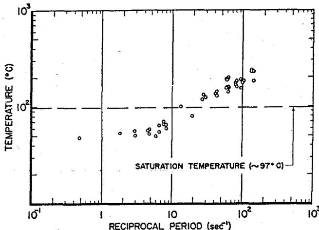
FIG. 16. Fuel plate surface temperature at the time of maximum reactor power as a function of reciprocal reactor period. Thermocouples were located at horizontal center line of reactor core in a central fuel assembly.
