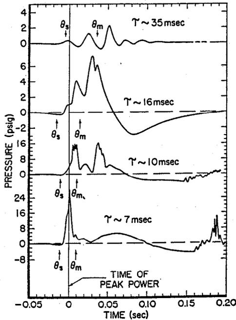
FIG. 11. Idealized transient pressure shapes for four reactor periods.  $\theta_s$  and  $\theta_m$  indicate approximate times at which fuel plate surface temperatures reached saturation temperature and maximum, respectively.
