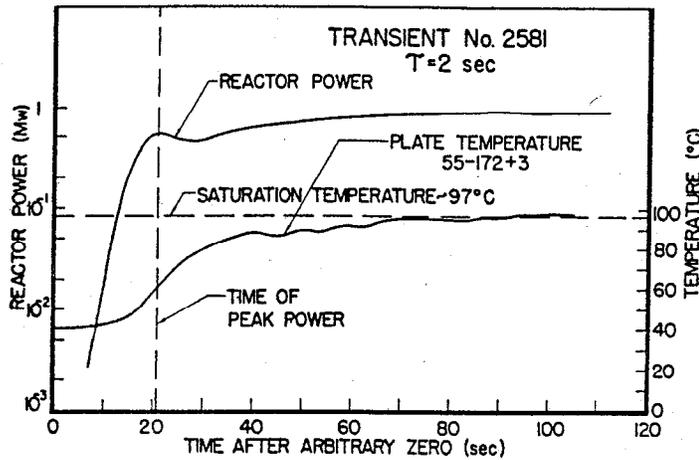
FIG. 4. Representative behavior following 0.48% reactivity addition ( $\alpha = 0.5 \text{ sec}^{-1}$ ).
