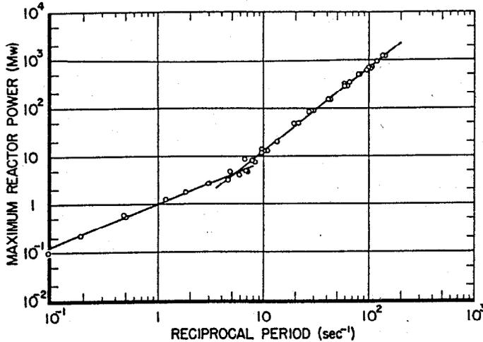
FIG. 12. Maximum reactor power as a function of reciprocal reactor period.
