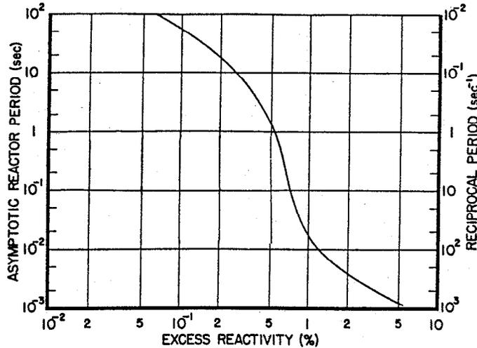
FIG. 3. Excess reactivity versus asymptotic reactor period (in-hour relation) for effective neutron lifetime of 50  $\mu$ sec using Keepin and Wimmitt delayed neutron data (7).
