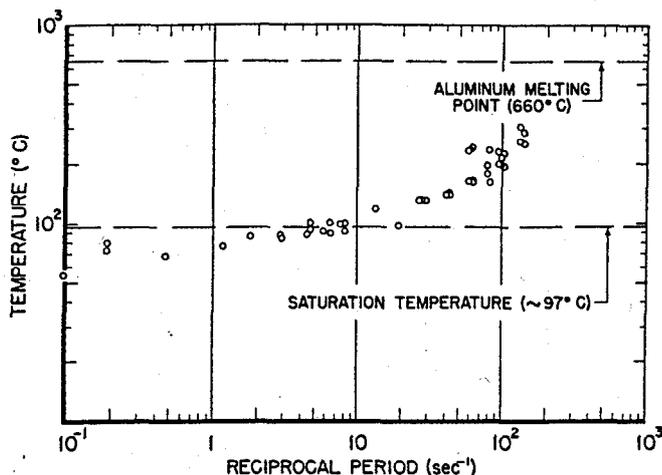
FIG. 15. Maximum fuel plate surface temperature as a function of reciprocal reactor period. Thermocouples were located at horizontal centerline of reactor core in a central fuel assembly.
