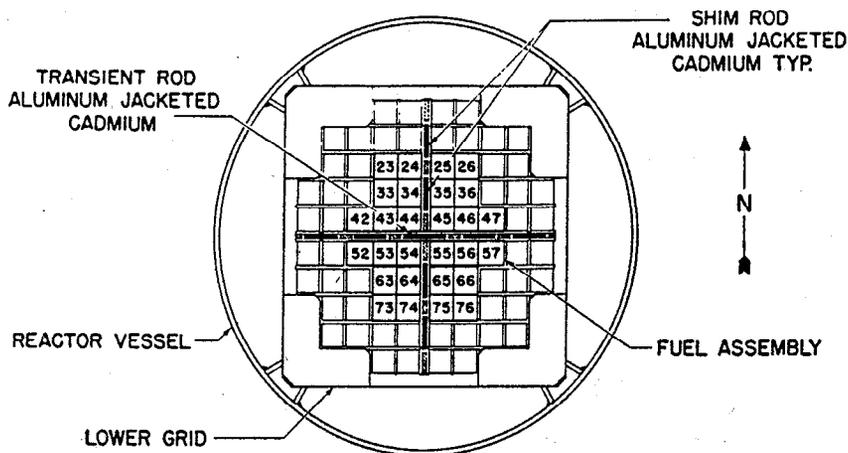
FIG. 1. SPERT I reactor core diagram showing lattice position numbering system.
