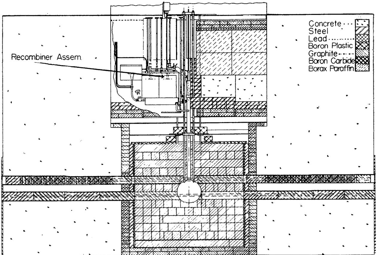
Figure 7. East-west vertical section of water boiler (Supo model)
