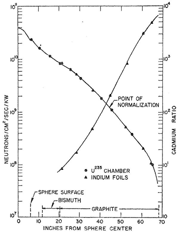
Figure 14. Supo north thermal column
