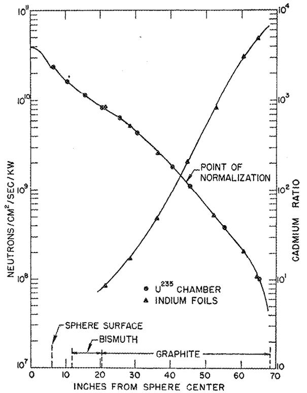
Figure 14. Supo north thermal column
