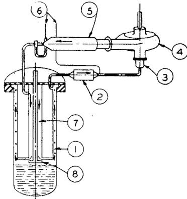
Figure 26. Schematic gas system: (1) spray condenser; (2) steel wool entrainment trap; (3) flow meter; (4) centrifugal pump; (5) catalyst chamber; (6) sampling tubes; (7) reflux condenser; and (8) solution baffle
