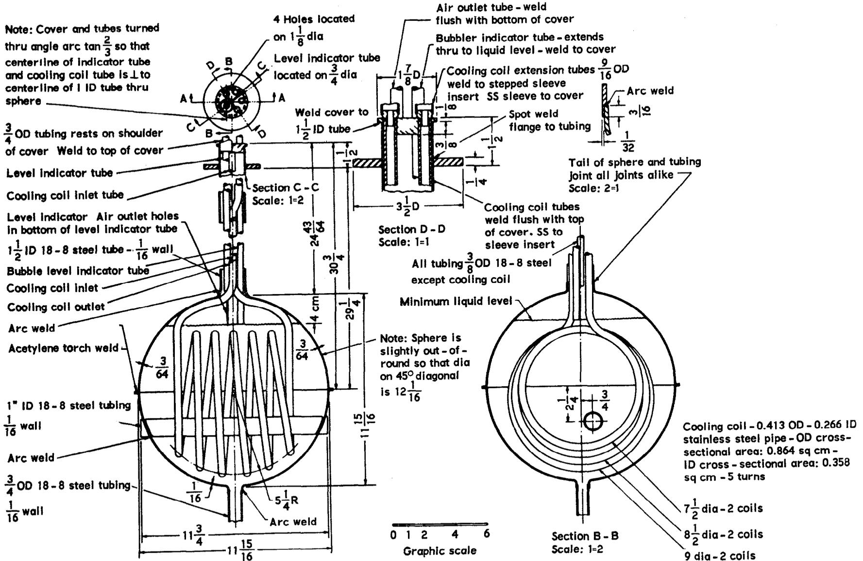
Note: Cover and tubes turned thru angle arc  $\tan \frac{2}{3}$  so that centerline of indicator tube and cooling coil tube is  $\perp$  to centerline of 1 ID tube thru sphere
