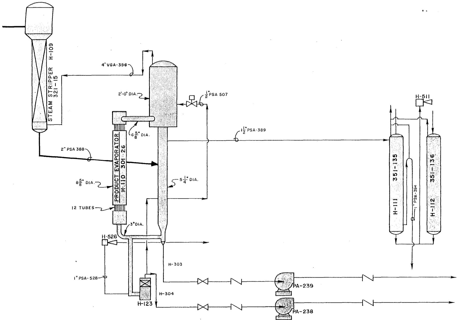
H-CELL PERTINENT EQUIPMENT - FLOW DIAGRAM
