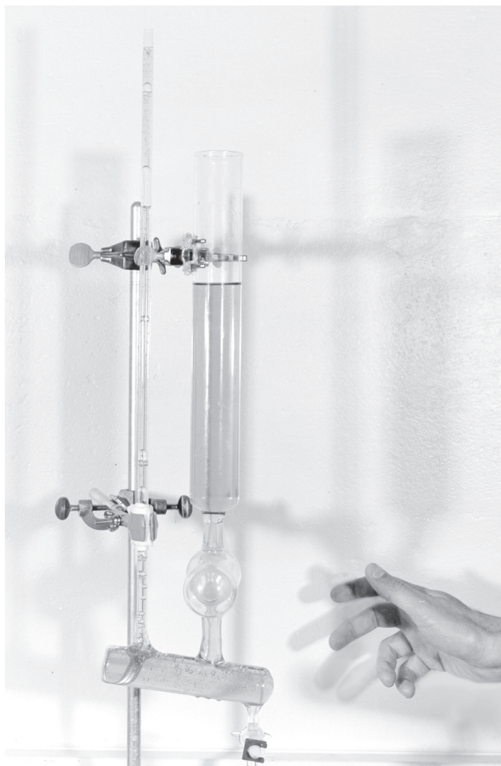
Fig. 108. A glass model of the experimental apparatus clearly demonstrates the accident phenomenon. The large diameter tube represents the central column sitting on top of a single simulated SCRAM valve. The vent to the SCRAM Tank, at the bottom of the photograph, is represented by the smaller diameter vertical tube. Colored water in this demonstration clearly shows the liquid being broken up by large air bubbles.
