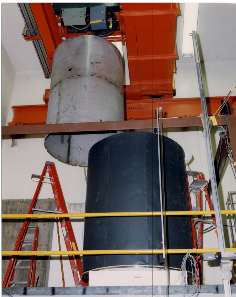
Fig. 129. Stainless steel, thin, cylindrical sleeves were used as “reactivity shims” in the Shielded Annular Tank program. Improperly moving one which had been immersed in high concentration fissile solution had caused wide-spread contamination of personnel and equipment. This occurred February 14, 1987. This photograph shows a different-but-similar shim before it ever became contaminated about to be lowered into the tank. The upper part of this figure was also used earlier to illustrate another feature.
