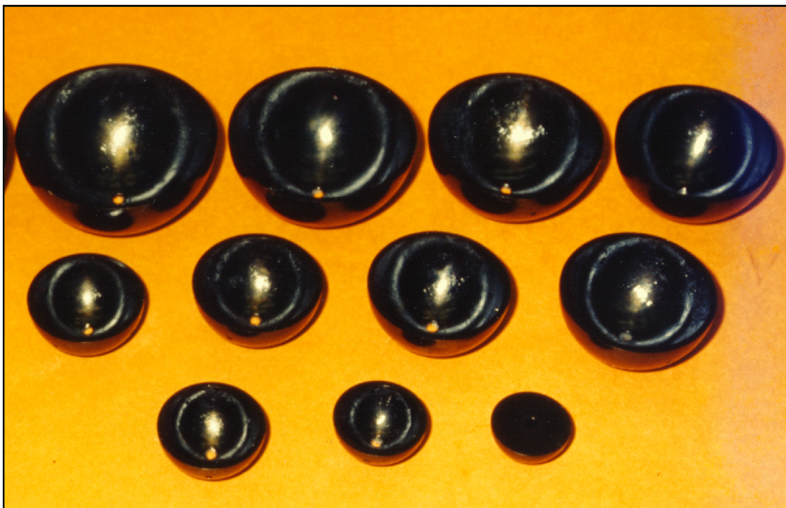
Fig. 91. Eleven of eighty nesting enriched uranium hemispherical shells are shown. Even-numbered shells could form one hemisphere; odd-numbered, the other. Shells were black in color because of an oxide coating; and they were shiny because of a thin coat of grease used to control contamination.
