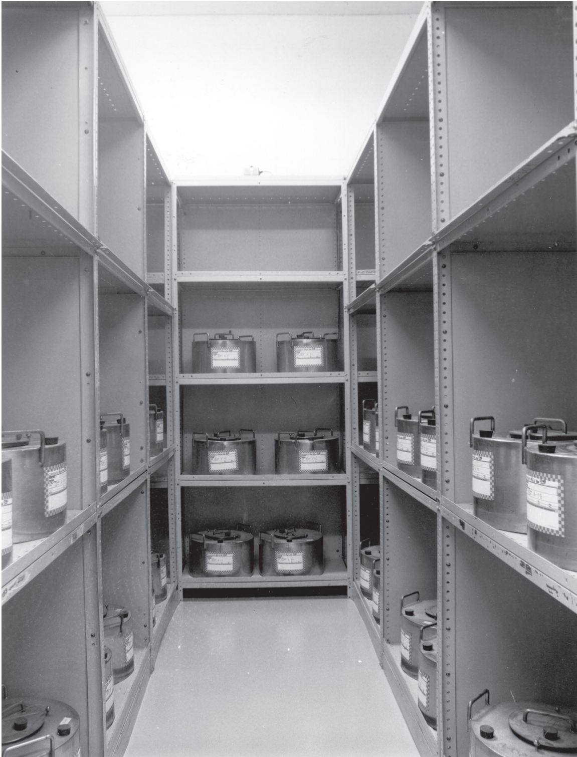
Fig. 36. Room 102 was used to store containers of solid fissile material on several sets of shelves similar to this U-shaped bay. The water-filled stainless steel containers seen here housed one doubly-canned plutonium machined metal cylinder each. Other shelves housed machined enriched uranium metal hemispherical shells in modified commercial pressure cooker pots as well as cubical cans of low-enriched compacted uranium oxide. Neither the pressure cookers nor the oxide cans are shown in this figure.
