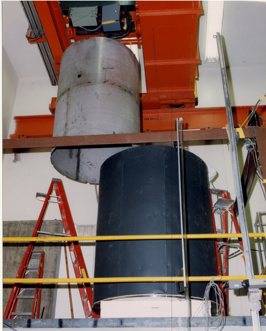
Fig. 22. The overhead traveling crane appears in the upper half of this photograph. It was far enough away from any experiment as to have negligible influence on any critical configuration. The crane's lifting capacity was rated at about 4,500 kg.
