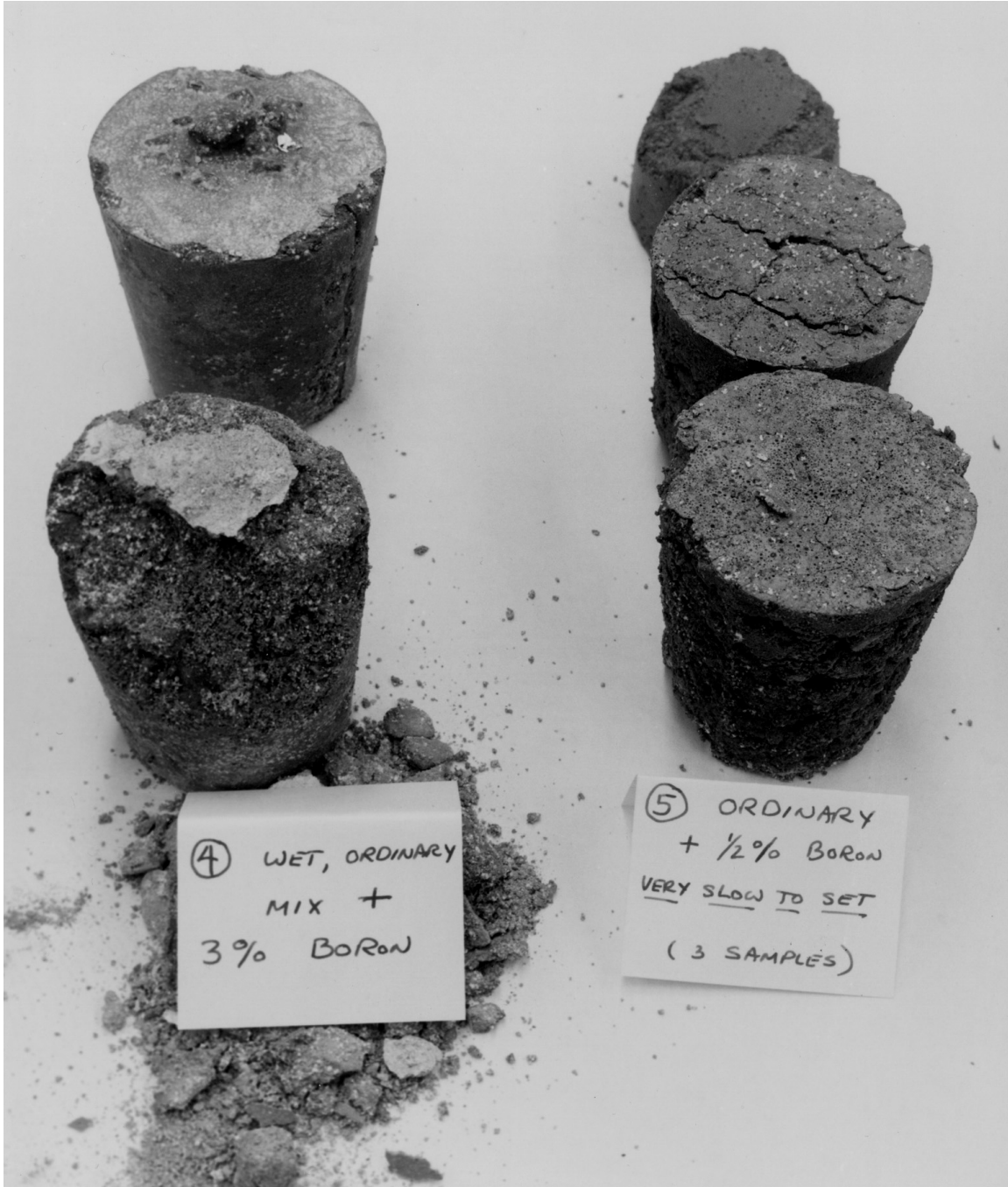
Fig. 117. An attempt was made to cast boron-loaded concrete substituting boron oxide for some of the sand (silicon dioxide). Test samples in paper cups did not work because boron oxide and water form boric acid which changed the pH of the mixture. They had no strength whatsoever; the mix at the lower left had 3% boron and could not even maintain its shape.
