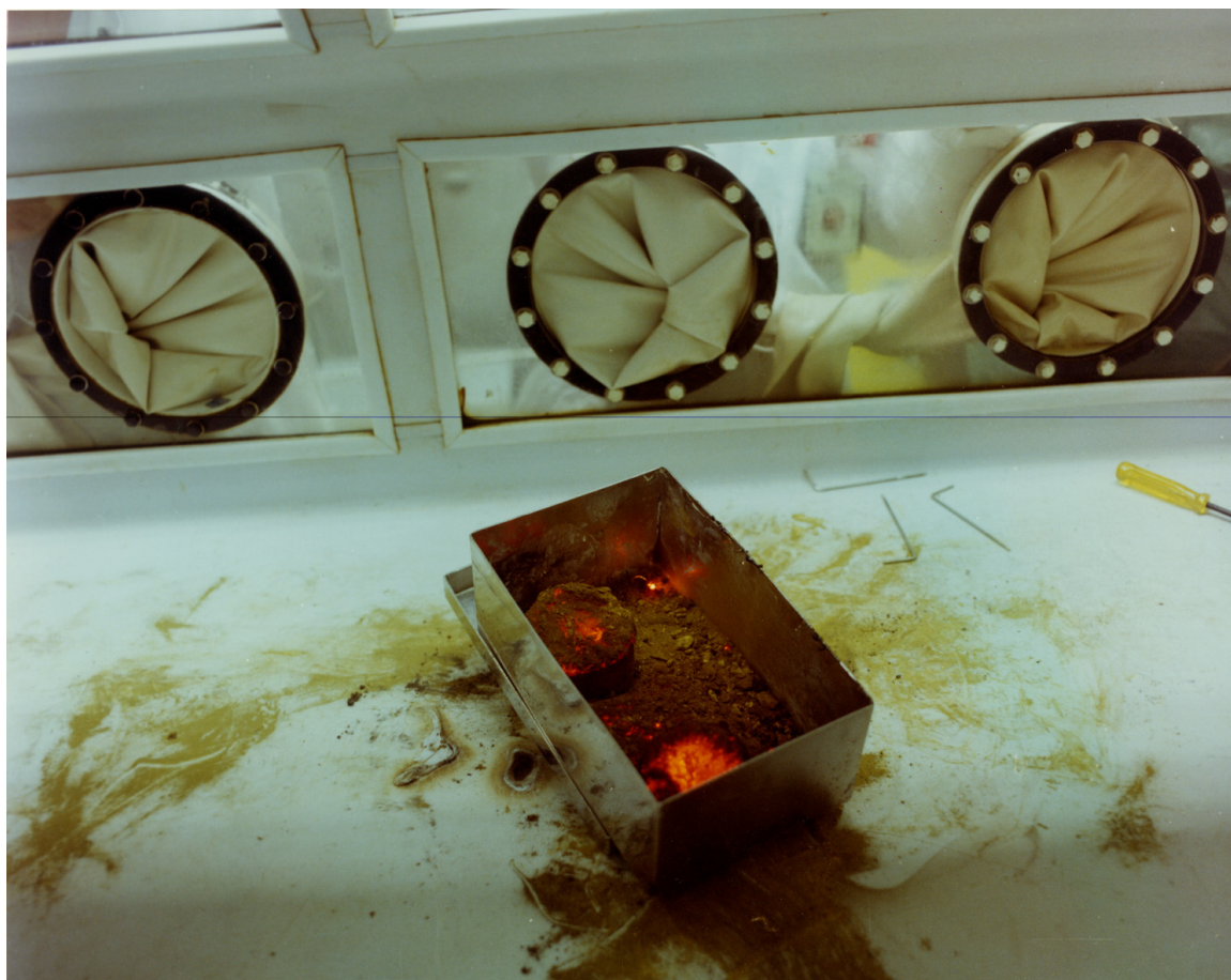
Fig. 127. One plutonium cylinder was uncanned in a Rocky Flats laboratory. The glovebox selected for this operation unknowingly contained an air atmosphere. In short time, sparks began to be emitted from the surface of the now-bare plutonium. The entire cylinder turned a dull red within a few minutes which allowed time to introduce a metal box with a layer of sand in the bottom. The cylinder was placed on the sand and allowed to combust completely. It looked like a glowing charcoal briquette at the stage shown in this January 19, 1983, photograph.
