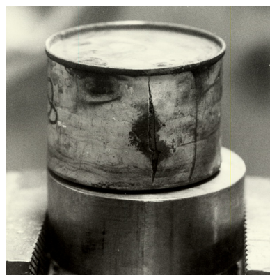
Fig. 124. Some plutonium cylinders showed evidence a similar event was imminent. This can's side wall had split open; but no oxide had yet filled the secondary container. This photograph was taken February 24, 1983.
