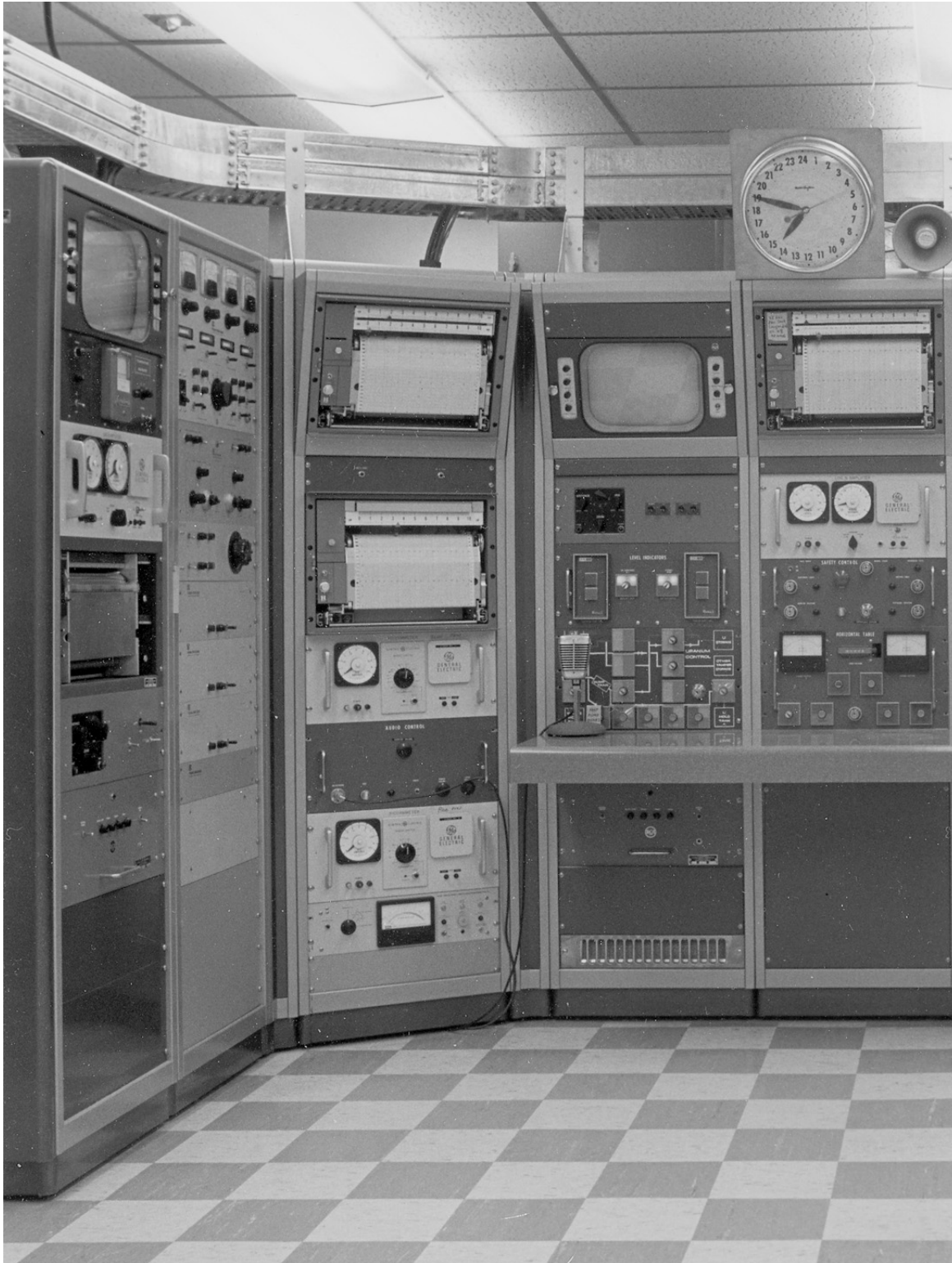
Fig. 70. The Control Console was situated in the south half of Room 112. Almost all critical and critical approach experiments were controlled from this location. The few exceptions were configurations assembled by hand using the in situ technique. This January 1969 photograph shows the console after the addition of two pair of chassis racks on either side of the original six racks.
