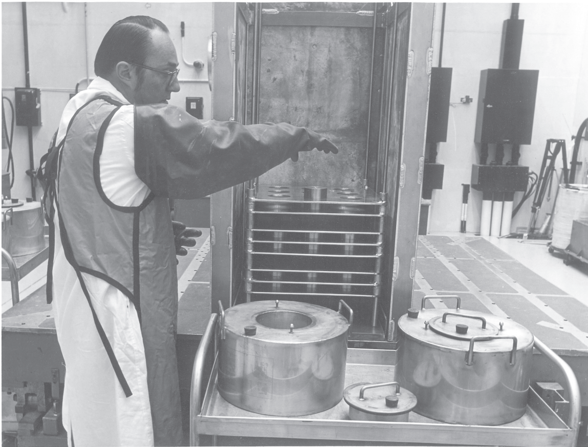
Fig. 101. The author is properly dressed for handling canned plutonium metal containing a considerable amount of Americium because of its age. Older plutonium becomes a strong gamma ray emitter. The glove and apron contain lead yet remain flexible. His film badge is worn inside the apron and the wrist badge under the glove. A half-mask respirator (not seen) hangs from his neck with the face seal against his chest. Glasses are safety glasses. Storage containers (foreground) for the plutonium are water-filled and lead-lined inside. Over 60 kg of plutonium have been assembled behind the three-sided shield in the middle of the photograph.
