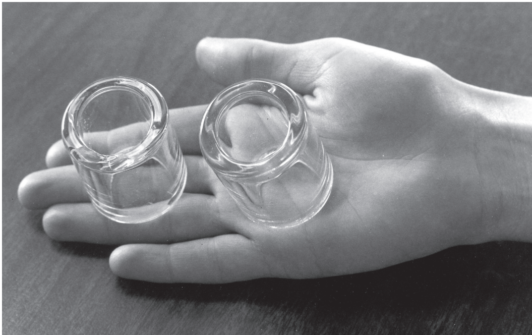
Fig. 98. Raschig Rings are small, right circular, cylindrical, shells of borosilicate glass. The glass contains about 12.6 % boron oxide. Boron effectively absorbs neutrons preventing criticality. Modern rings since 1970 are tempered for strength and fire polished on the ends. The hand belongs to this author's Secretary for a quarter century, Carla Fisher.
