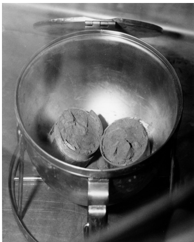
Fig. 126. Some plutonium cylinders had been so badly corroded by water vapor they fell in two during the uncanning operation. This photograph was taken January 20, 1983.
