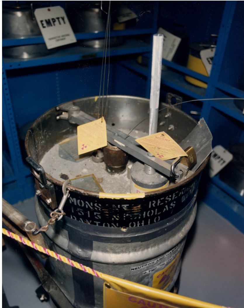
Fig. 40. The “source pig” was a small drum filled with paraffin to moderate neutrons and wrapped with cadmium sheet to absorb them. Four neutron sources exist at the ends of the wires shown emerging from the pig. The lead cylinder at about 5:00 o’clock housed a gamma ray source. Square paper tags contained information about each source. The pig was on wheels for easy movement but normally remained in Room 102.
