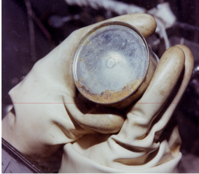
Fig. 125. Some inner containers showed evidence they had been in contact with moisture; but that water had not yet penetrated. Because of the mechanical seal between aluminum can and steel lid, an eventual problem would have been almost a certainty. This photograph was taken January 20, 1983.
