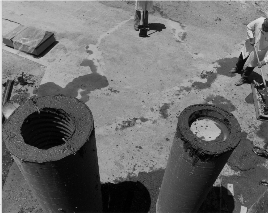
Fig. 118. Boron-loaded cylindrical “plugs” were successfully cast using an inert boron-rich mineral instead of boron oxide. The mineral replaced aggregate instead of sand. Many were cast in different outside diameters and different radial thicknesses. They were cast at three nominal boron concentrations (0%, 1% and 3%) and of two earthen materials: concrete and plaster. These two concrete plugs have just been poured. One used a steel culvert as the central form.
