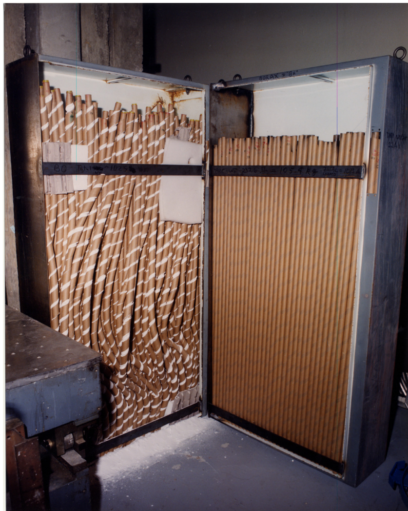
Fig. 128. The Poison Tube Tank was to have used a number of different neutron absorber materials. Some of these were solid; but some were powders and had to be contained. Long, thin paper tubes made of spiral-wound laminations formed that container. Several powders, such as borax, cadmium oxide, and others worked well as witnessed on the right side of this photograph. Boron oxide did not. The material is hygroscopic; and absorbed water caused the tubes to weaken and unwind as shown on the left.
