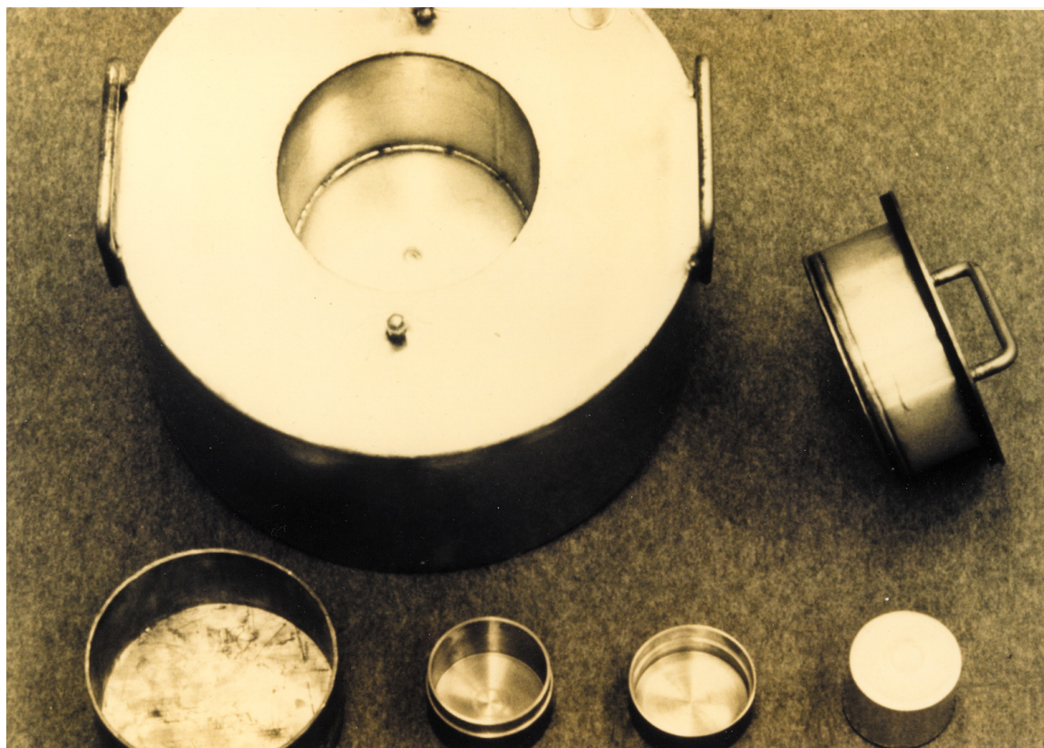
Fig. 97. The storage pot for plutonium metal cylinders was a water-filled and lead-lined “donut.” Water filled the pot (top left) and the lid (right). A lead insert (lower left) slipped inside the pot; and the bottom of the lid was lead covered as well. The aluminum-canned plutonium metal cylinder (lower right) fit loosely into the thick-walled stainless steel outer container (bottom center).
