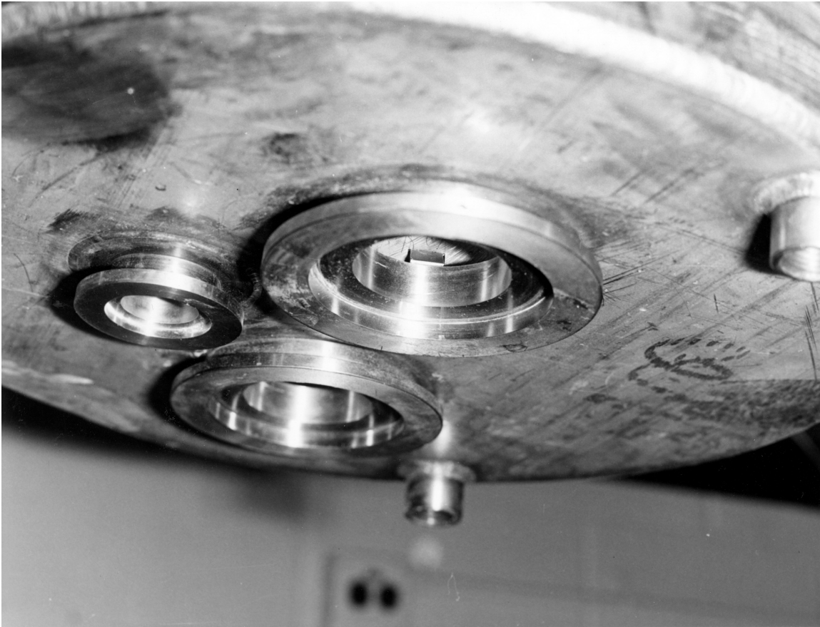
Fig. 24. The smaller Marmon coupling connected the experimental tank to the FILL/RETURN line. The two larger-diameter couplings similarly connected to the pair of SCRAM valves. This is the underside of some small-diameter experimental tank.
